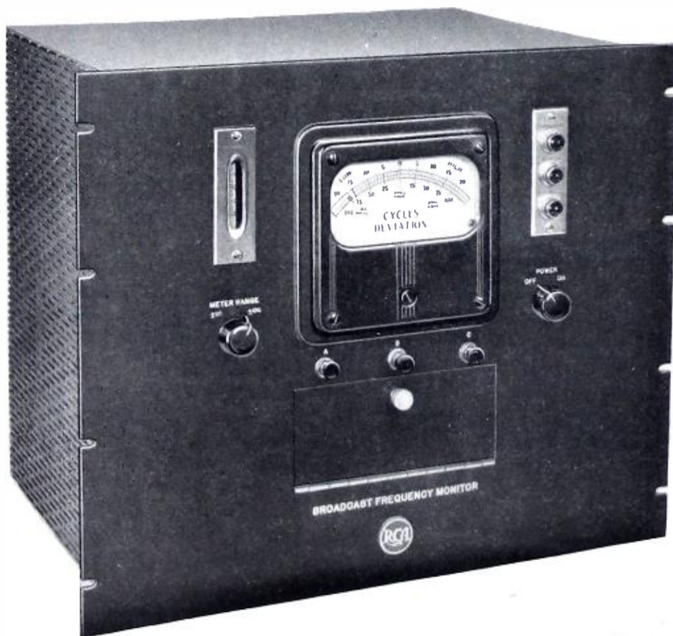
Front panel view of the 311-A Frequency Monitor.
