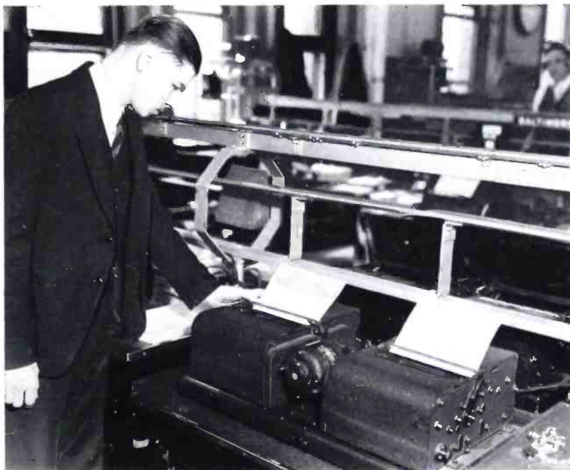
(Above) Facsimile receiver employed in RCA ultra-short wave radio circuit connecting New York and Philadelphia.
