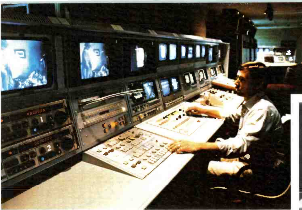
Master Control Console (left and below) provides complete machine controls for operator, and a direct look-in at the 110 kW transmitter operation.
