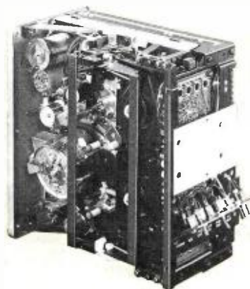
HR-1 with cover removed. Compact design with fewer moving parts improves reliability and performance.
