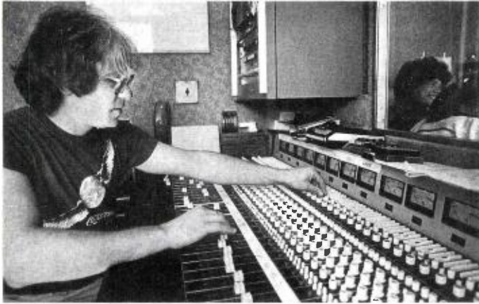
Audio Console on StarTruck (above) can handle 44 inputs and has a 24-channel output.
