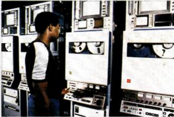
TH-200 VTR's with Dynamic Tracking are used for both program playback and production.
