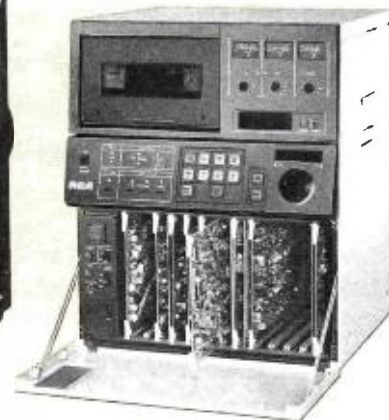
HR-2 Studio VTR, with lower panel dropped, showing front access to plug-in modules.
