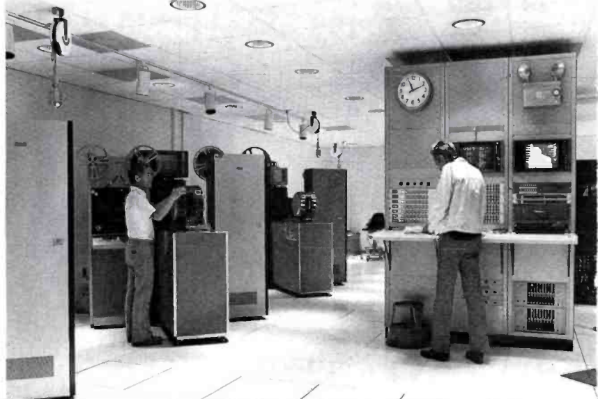
Telecine and Videotape room. The Control/Monitoring station at right identifies delegated and assignable videotape and film sources to provide for effective machine utilization without disrupting on-air operations.
