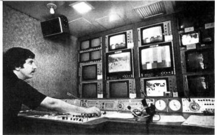
Audio Console on StarTruck (above) can handle 44 inputs and has a 24-channel output.
