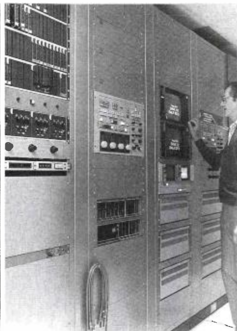
TK-47 Camera Set-Up Terminals and Camera Processing Units are rack-mounted in the Master Control area.
