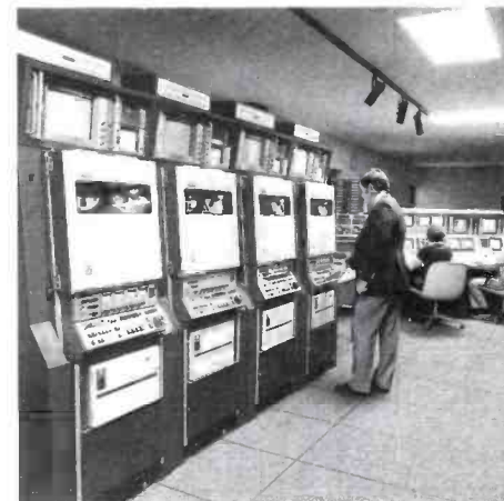
Two of the four TH-200 VTR's at WCLQ-TV are used for program playback and two are primarily production units. All are equipped with Dynamic Tracking.
