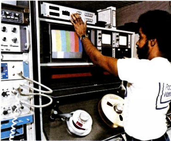
Each tape machine has its own input selector and can select any output from the routing switcher. The result is virtually unlimited flexibility in utilizing equipment.
