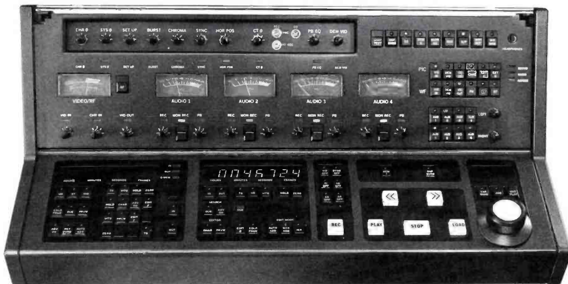
Machine controls for TR-800 are centrally grouped for operator convenience.
