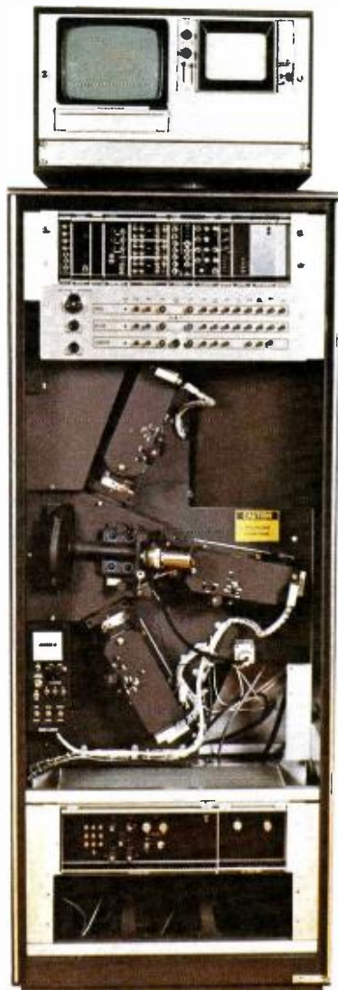
Inside the TK-29C, with the door removed.
