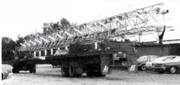
WITN's Circularly Polarized TBJ Panel Antenna stands tall (left) after its long truck ride from RCA's Gibbsboro, NJ antenna facility. (Below)
