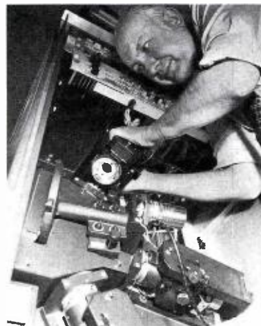
New precision yoke assembly for TK-29 Cameras.
