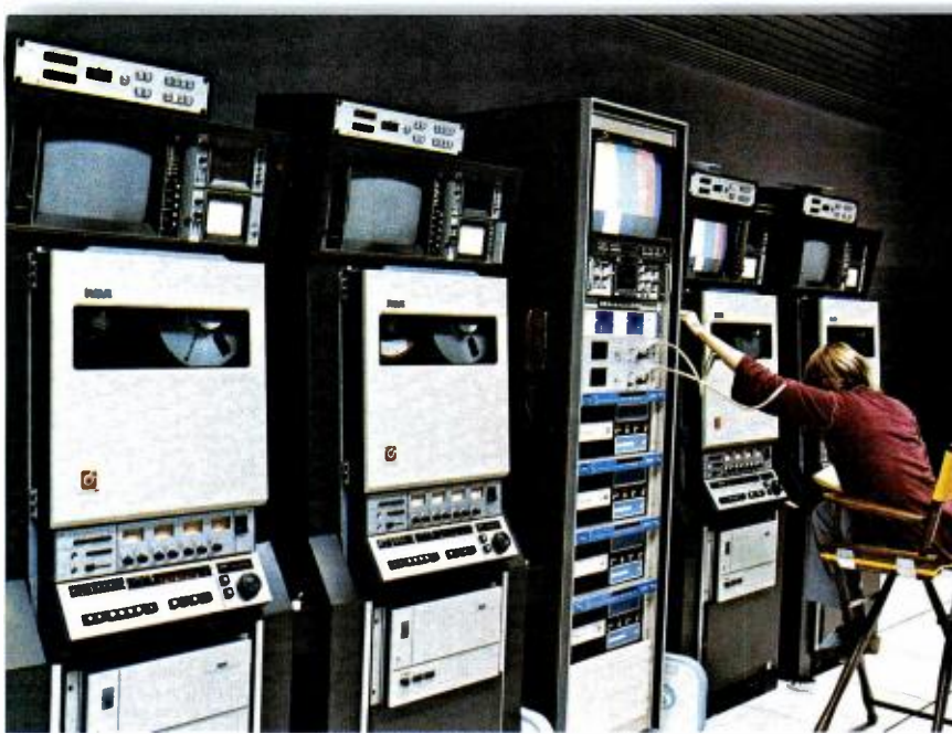
Four TH-100 one-inch VTR's in a separate group are used as auxiliary playback machines.
