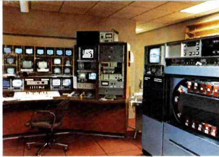
Another view of MC. The TCR-100A at right is used for airing commercials.
