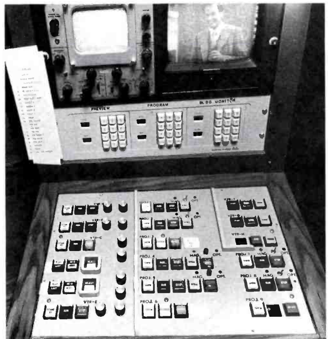
Remote machine control panels were custom-designed by the TV-10 technical staff.
