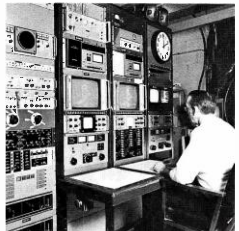
Status interface panel in open position. At bottom is a fuse panel through which all metering inputs are routed before passing into the system.
