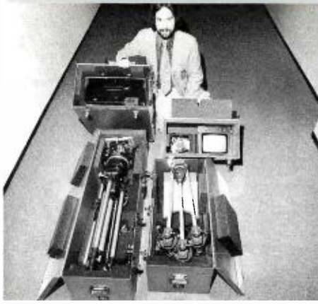
For location work, Quaker ships their TK-630 cameras in special foam-padded aluminum cases. Picture sequence (left) shows one of the cameras being packed for shipment.
