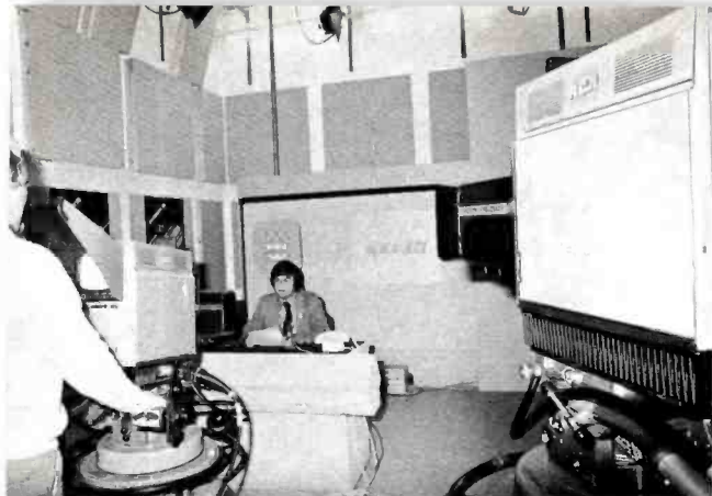
(Top left) One of four production studios for interviews and comments. Each of three studios used a pair of TK-44's. Two more RCA cameras were available on an assignable basis.
