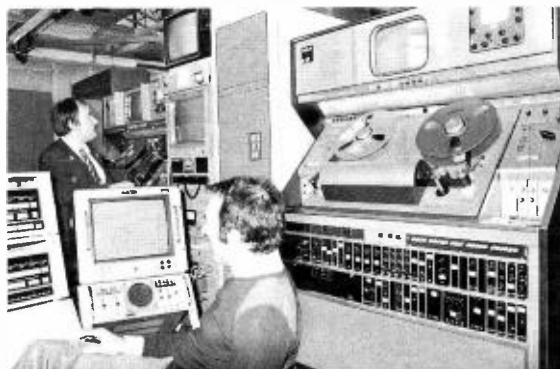
ORF utilized twelve TR-70C's in producing the world program. Four were located in two OB vans. The rest were assigned to four editing suites in which action highlights from many hours of recorded material were quickly assembled. The two machines shown here operated at half speed and were equipped with dual-cue programmer editing systems.
