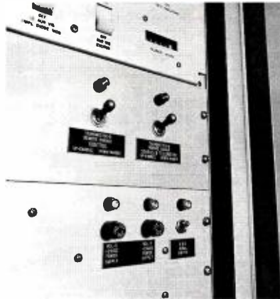
Monitoring and status displays for KNTV transmitter operation. Lower panel is logic system for RF switching sequences. The panel above this displays the "Summation of Control Data" referred to in text.
