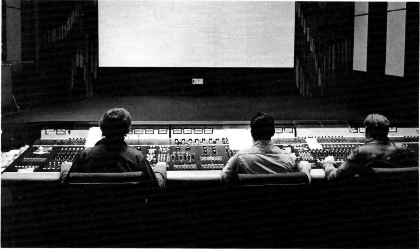
TBS' Dubbing Five re-recording stage from behind the mixing console. Display panel beneath screen is a footage counter.
