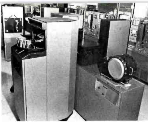
Latest additions to KY-3's technical area are two TK-28 telecine islands, one equipped with a TCP-1624 Cartridge Film System (foreground).
