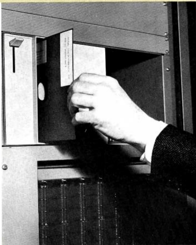
Magnetic "floppy" disks are used for message storage. Memory is random, so any message in storage is available at any time. Each disk can handle 3070 addresses.
