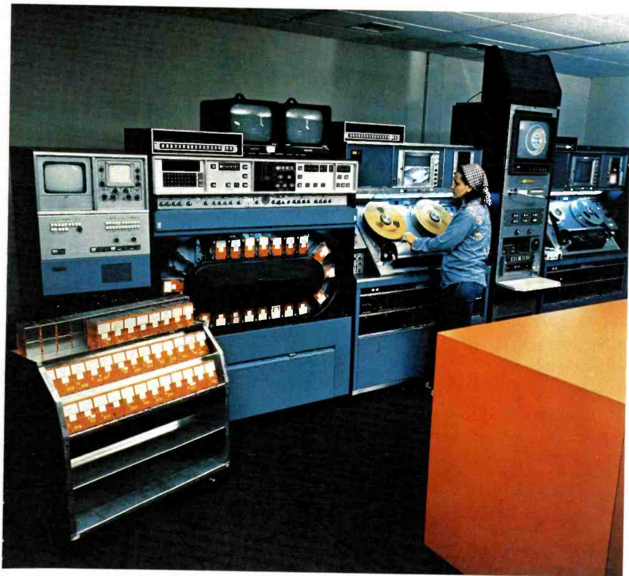
Adjoining Master Control is the Video Tape Room, with its complement of three TR-70's, editing facilities, and two TCR-100 cart machines.
