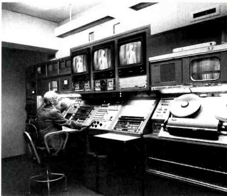
Four TCR-100's are installed, two in a bay, with complete monitoring facilities. Machines are loaded from carriages which bring scheduled carts from storage area. With 8,000 "carts" on hand at NBC Burbank, storage and cataloging systems are critical. Rolling shelving provides ready access to stored carts.
