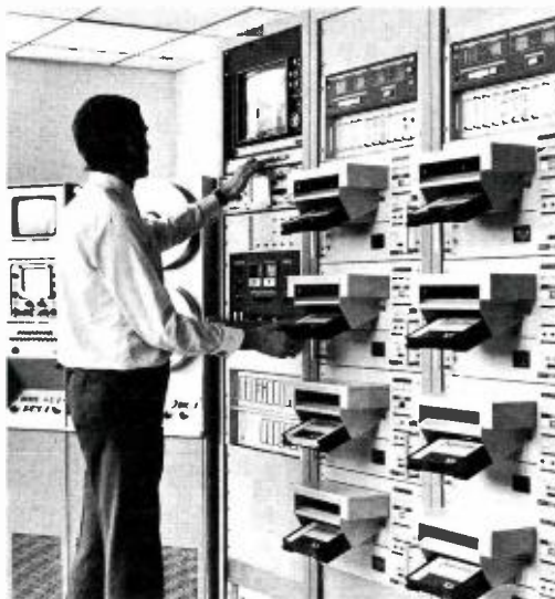
Cassettes are produced in quantity from 2-in. video tape masters played back on the TR-60 quadruplex VTR. A TR-70 is also used as head equipment.
