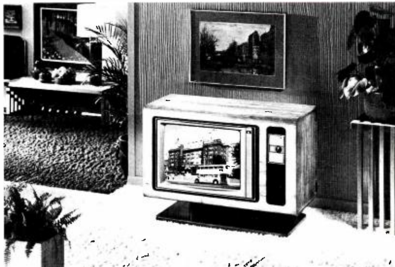
RCA's MOST AUTOMATIC COLOR—Ball games in the afternoon will be easier on armchair TV viewers with the development of a new ColorTrak television system by RCA that among other advances, automatically adjusts picture brightness to room light and maintains picture contrast at the TV set to prevent fading, thus avoiding washed-out pictures.
