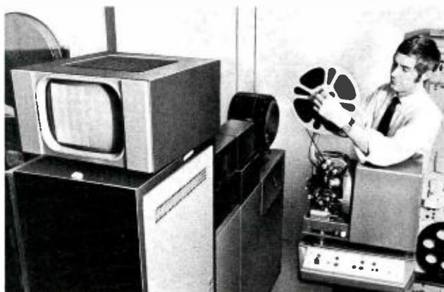
A TK-28 telecine chain allows insertion of film or slide material to the cassettes. It has super-8mm, 16mm and 35mm film projectors plus a 35mm slide projector, and is also employed for a very active film-to-tape transfer service.
