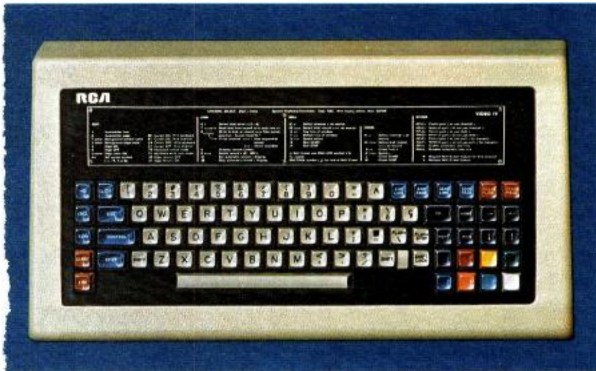
This standard keyboard is the most frequently used Video IV input. Up to four may be used with each system.
