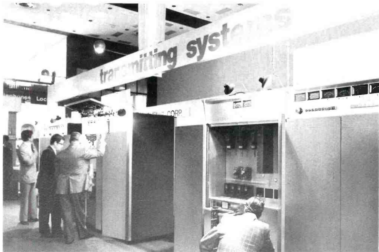
Three in a row. The TV Transmitter line-up at NAB included the TT-25FL lowband, the TT-25FH highband VHF systems, and the TTU-30C UHF which is solid state up to the final stage.
