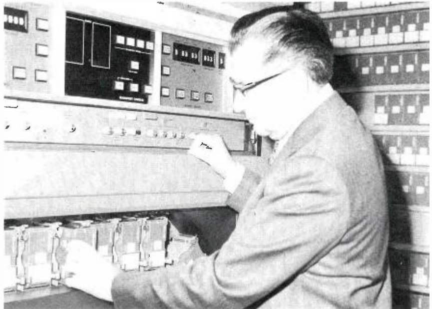
Ted Wadson, Director of Engineering at Edmonton's CFRN-TV, loads the station's new TCR-100 Video Cartridge Recorder with commercials and other station break material. Mr. Wadson says that use of the RCA "Cart" machine has "significantly reduced errors during breaks and resulted in fewer makegoods",
