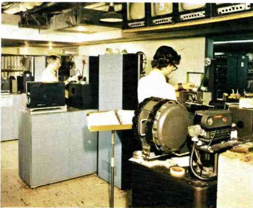
TV's technological growth is displayed in this grouping of past and present WGAL film and tape sources. Shown are the contrasts between early monochrome and modern color film islands, along with those of early low-band and contemporary high-band tape machines.
