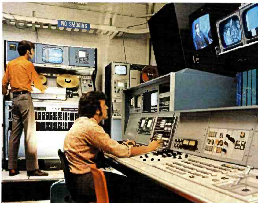
Time Code Editing provides frame-accurate editing, expanding the capability of the two-camera studio. Tapes are planned to take full advantage of the editing system to make a more interesting end product.
