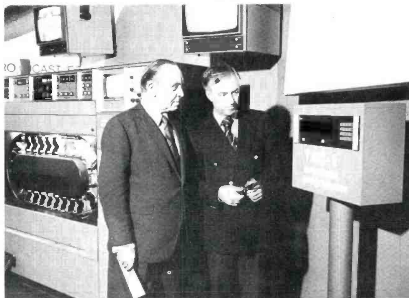
As many as 80 program segments can be sequenced automatically with the new TAC-1 Automatic Programmer. Sources can be tape, film or slide.
