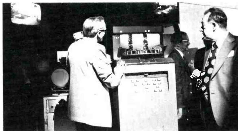
A major attraction at the show, the TCP-1624 can handle up to 24 film cartridges on a carousel tray. This unique system can broadcast a single spot or a sequence of spots in any combination, from 10 seconds to two minutes.
