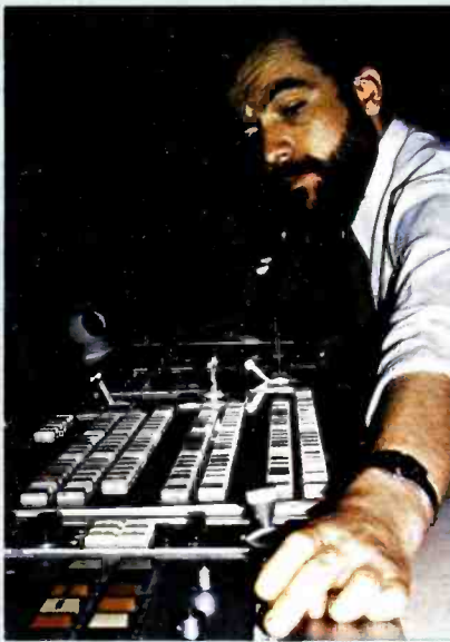
Rendezvous point for all camera, tape and telecine sources is the RCA TS-51 switcher. This video production tool creates visual effects.
