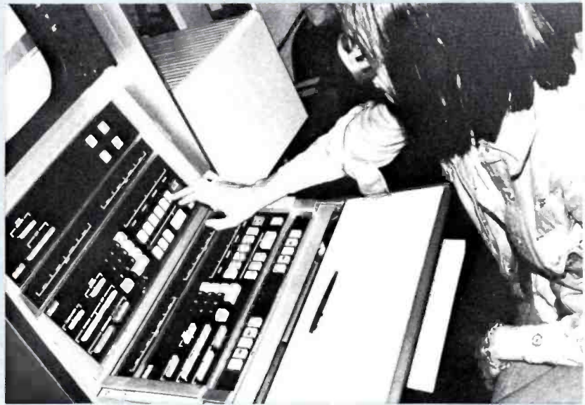
With the aid of RCA's Time Code Editor, VTR Supervisor Jacqueline Jeannert uncomplicates the video tape editing procedure. Identifying each frame of information in hours, minutes, seconds and frames, the TCE lends speed, accuracy and flexibility to the whole process.
