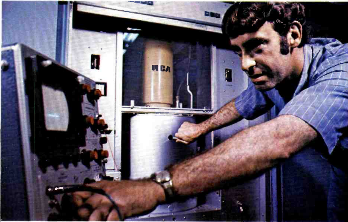
Carriage arrangement permits quick change of klystron when needed.
