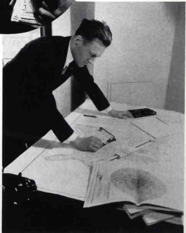
(ABOVE) MEASURING THE COVERAGE AREA OF A RADIO STATION BY THE USE OF A PLANIMETER
