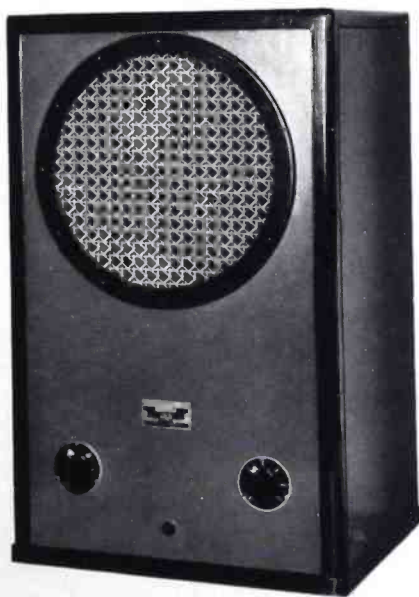
STATION HOUSE RECEIVER, EMPLOYED TO PICK UP SIGNALS FROM THE MOBILE TRANSMITTER
