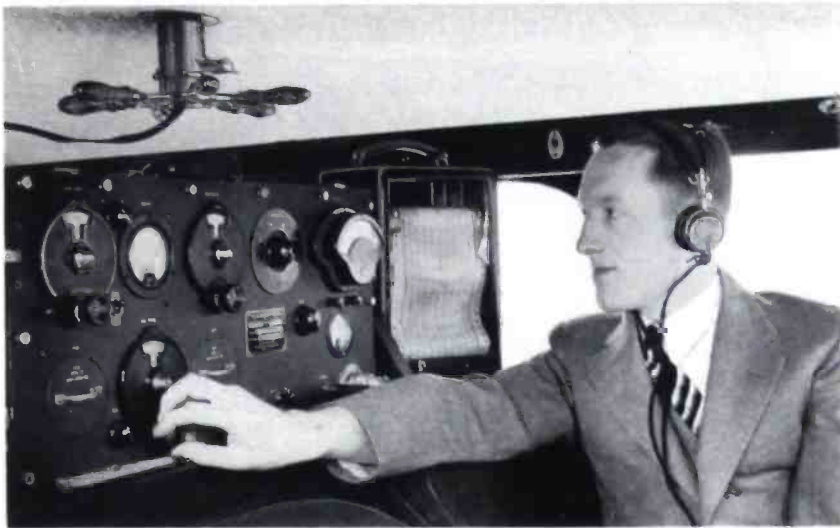
VIEWS INSIDE ONE OF THE NBC RADIO ENGINEERING CARS, SHOWING ONE OF THE FIELD SURVEY MEN OPERATING THE RCA TYPE 75-B MEASURING SET. THE GRAPHIC RECORDER MAY BE SEEN AT THE CENTER OF THE PICTURE, AND OVERHEAD IS THE WHEEL CONTROLLING THE LOOP ANTENNA
