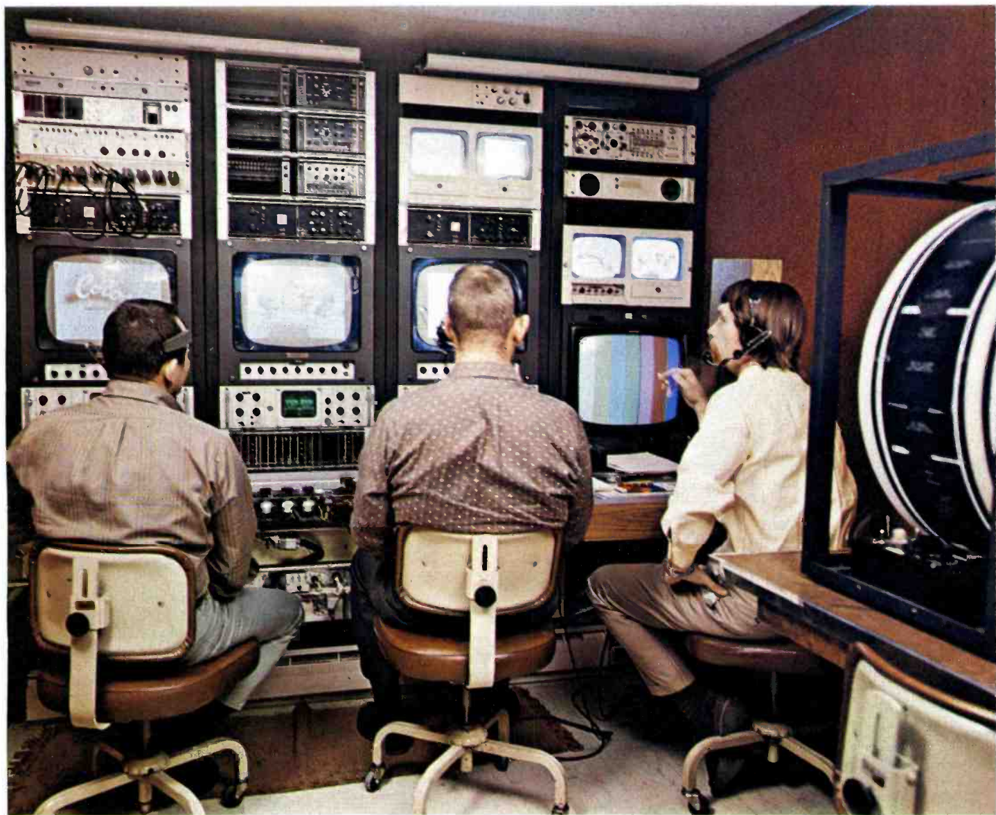
Video and production control for WLVT-TV is housed in mobile van unit. This control center is used for both remotes and studio operations.
