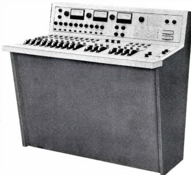
Custom console for KOMO color mobile unit handles 10 mikes and 14 high level inputs. Three mixer busses and three submaster controls combined into three output channels with one-by-two splitters. The console also includes ten-by-two switching matrix, cue, echo send and receive, foldback and output monitoring.
