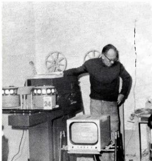
FIG. 6 Installation of film chain.
