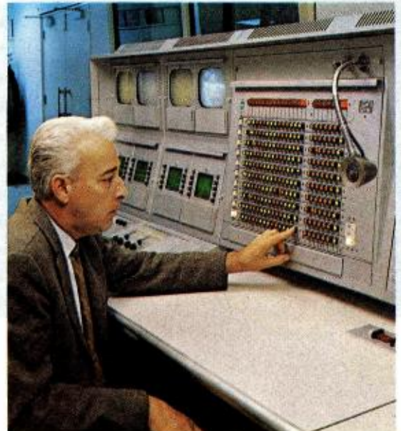
STATION BREAK AUTOMATION section houses TSA-3 panel capable of handling 15 video and 7 audio inputs in a preset sequence of ten events. Panel at the operator's right includes remote control of sync generators and stabilizing amplifiers.
