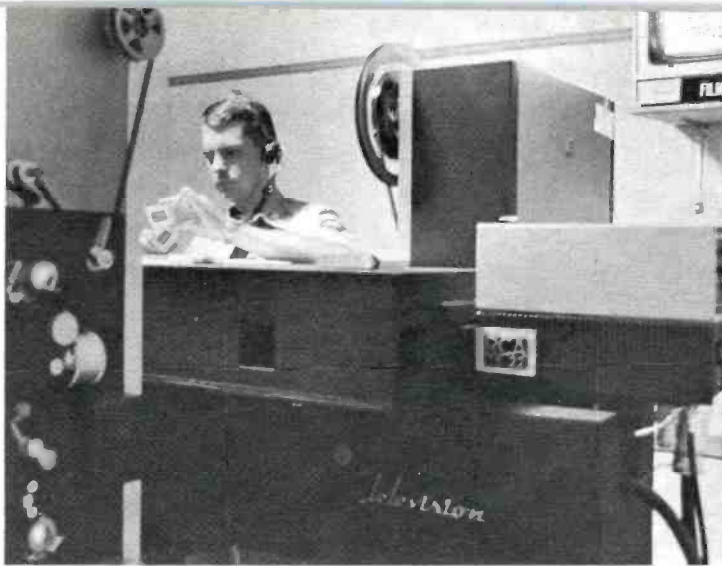
FIG. 7 An Army student prepares slides for a student newscast in the "new" film chain room. DINFOS recently "modernized" the telecine with two RCA TP-66's. The TK-22 remains a part of the system.
