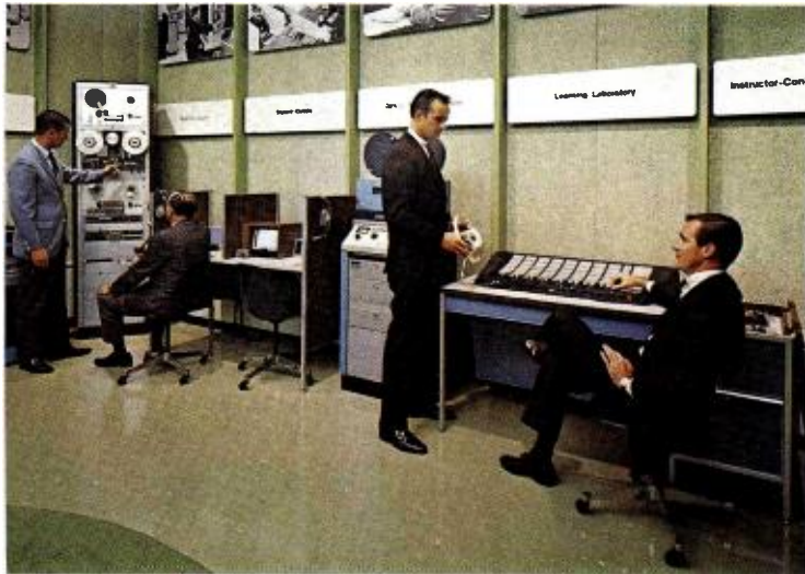
FIG. 3 Systems area contains (l. to r.) operating Select-a-Lesson information retrieval equipment rack, student carrels, optical recording system, and learning laboratory. Not shown are a TeleRoamer mobile TV console and an instructor-controlled television system for classroom use.
