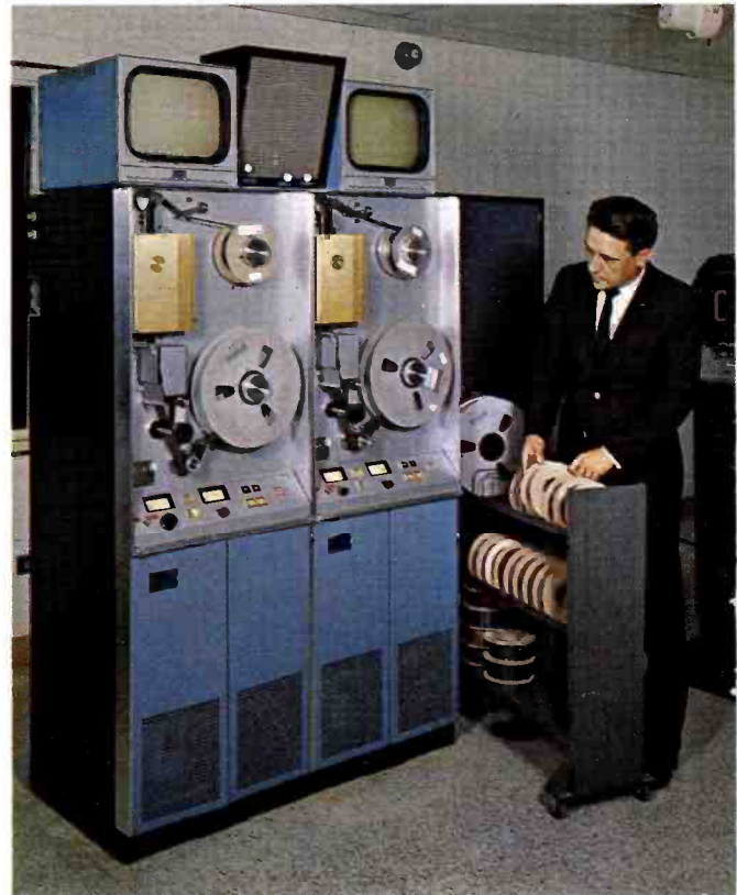
FILM AREA includes two film islands, storage and film editing facilities. Latest-design equipments for color and monochrome include a TK-27 4-vidicon color film chain and two TK-22 monochrome film chains.
