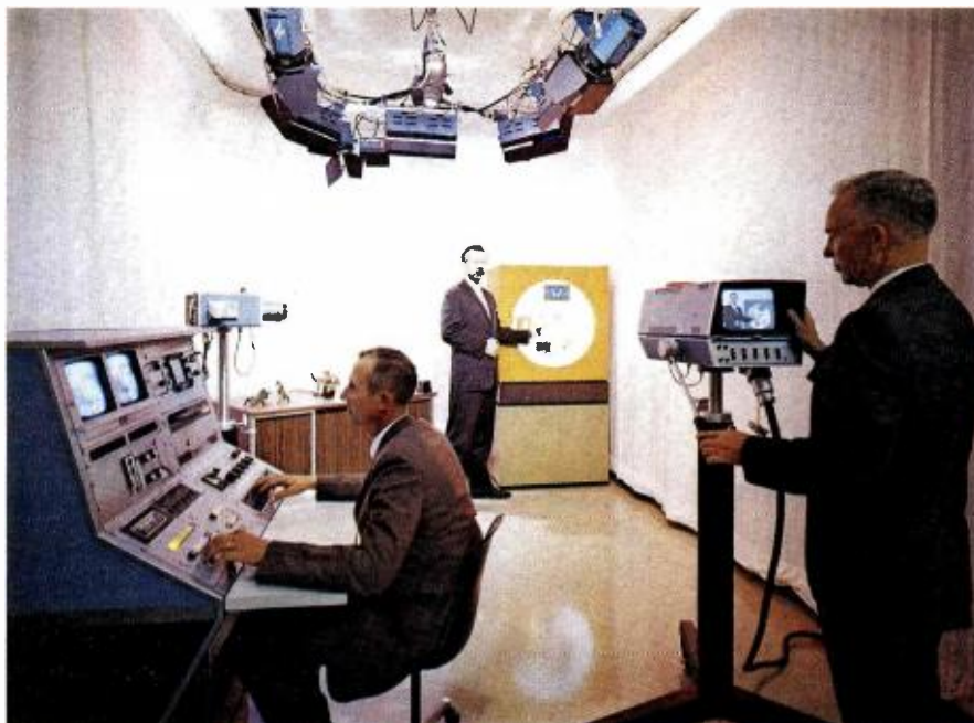
FIG. 2 Small TV studio contains complete facilities for camera demonstration and testing. Shown left to right are: PTC-2 console with PTS-1 switching system and special effects, camera controls, audio system, and monitors; PK-315 viewfinder camera; "animation unit" used in demonstrations; and PK-330 studio camera.
