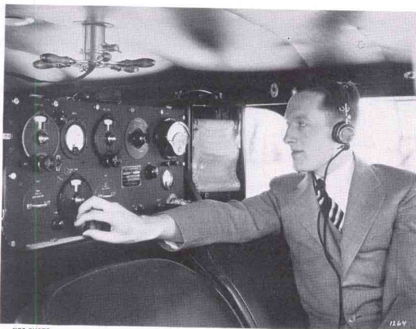
W. A. FITCH, NBC RADIO ENGINEER, USING THE RCA TYPE 75-A FIELD INTENSITY METER WITH RECORDER, IN THE NBC ENGINEERING CAR, No. 2 NBC PHOTO
