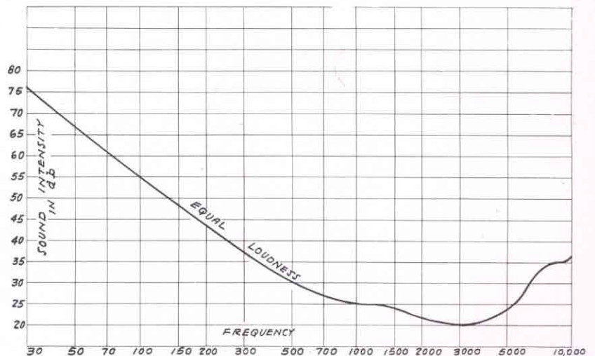
FIGURE 2—CURVE SHOWING SENSITIVITY OF THE EAR AT LOW SOUND INTENSITY
