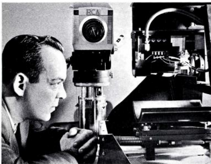
FIG. 1 New laser beam image reproducer is demonstrated by RCA engineer Dennis Woywood. The unit is recording by laser beam an image consisting of 5,000 TV lines on a 9 x 9-inch photograph plate. Such images are transmitted to the laser by a new "return beam vidicon" TV camera, shown in background, that produces pictures 10 times sharper than those provided by a standard TV camera.
