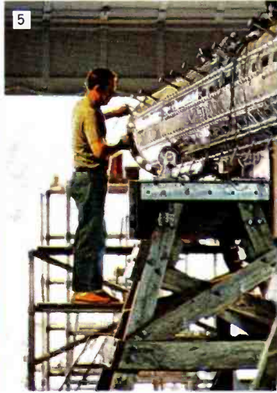
(5) Assembling one of the largest Pylon Antennas ever built. It will provide a base for a large Super Turnstile antenna in a stacked antenna arrangement.
