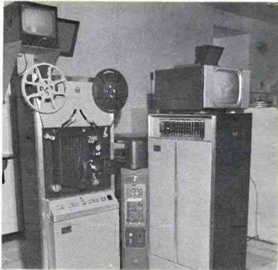
FIG. 8 CFTO employs the RCA Big-Tube matched color film system for all slide and film segments in their productions.
