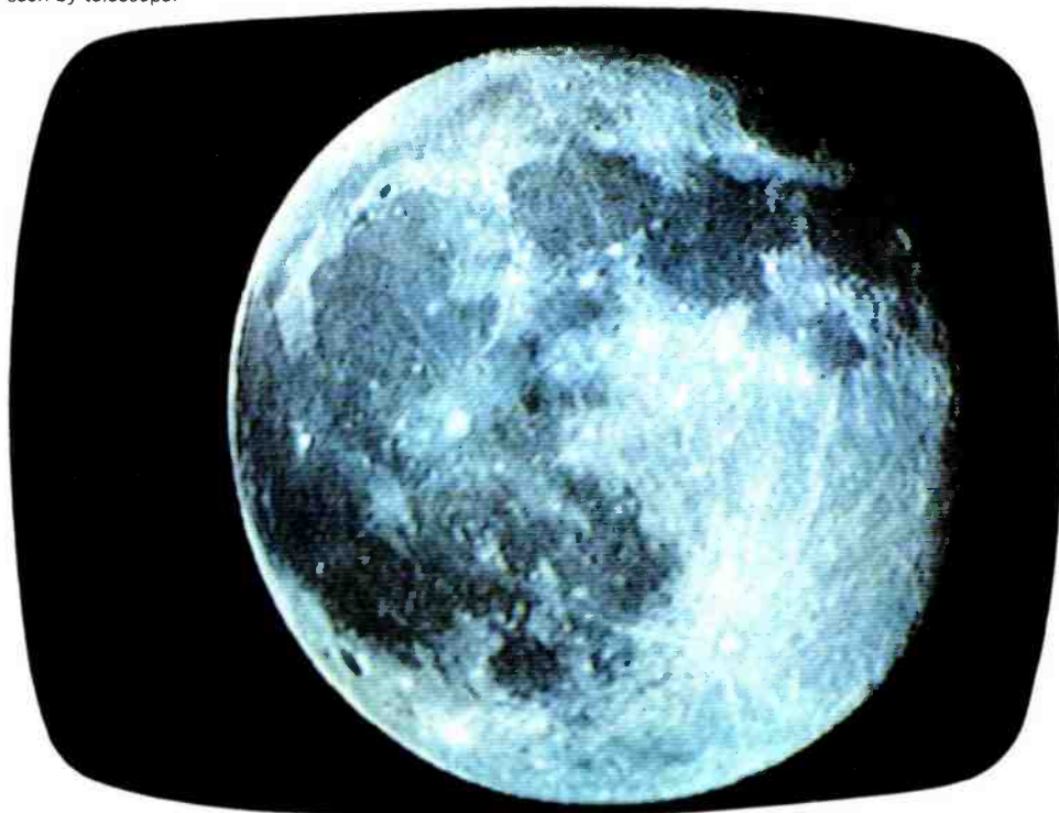
FIG. 5 A tighter shot with lens focal length of 110 inches. At this magnification, moon moved across kinescope at rate of 1 inch in 15 seconds.
