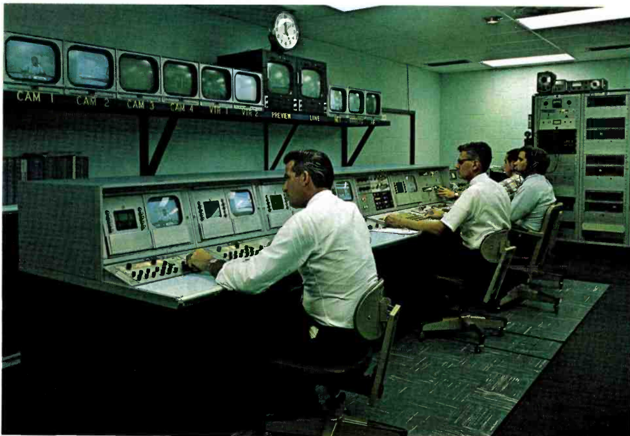
FIG. 7. Unified, New Look monitoring and control position comprising color studio and film camera controls, TS-40 switcher and special effects system, film remote controls, audio console and tape recorders.
