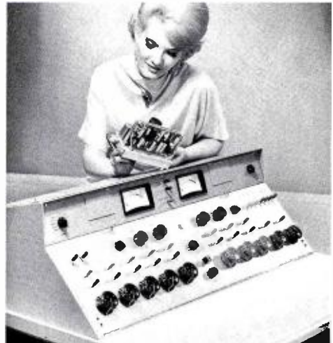
Plug-in chassis give flexibility to consolettes.
