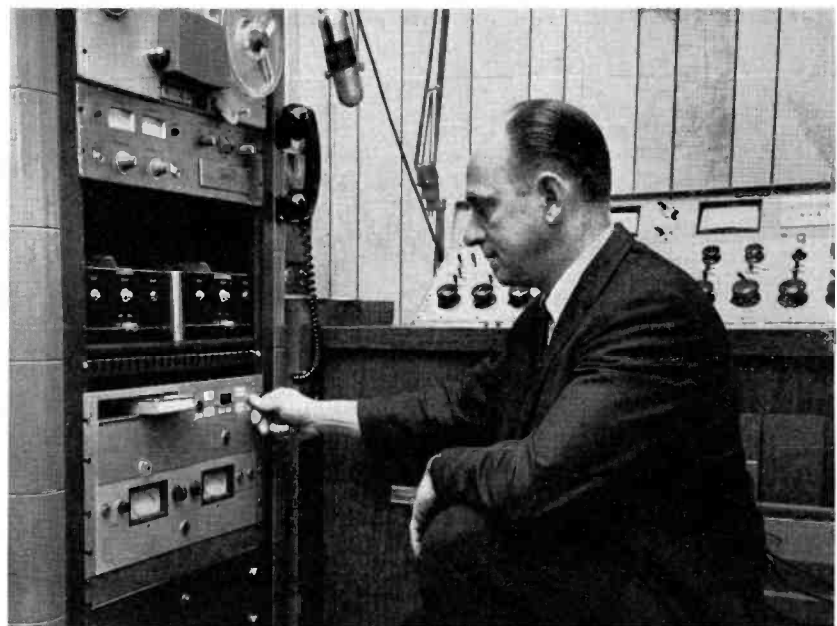
FIG. 5. Production control resembles the main control room in equipment complement and layout. Another BC-7 consolette is used, with the dual 77DX microphones for stereo pickup, stereo reel-to-reel cartridge tape equipment and a disc turntable (not shown). Although the room is designed primarily for production of programming, on-air operation is occasionally delegated to this console.
