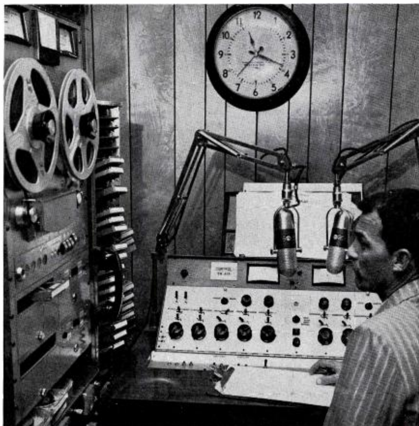
FIG. 2. Control room equipment includes the BC-7 stereo control console, two turntables (not visible) three cartridge tape recorders, two stereo reel-to-reel tape machines, two 77DX microphones for stereo announcements, remote extension meters for the BW-73 FM multiplex monitor and a transmitter remote control system. Gary Hoffman is the announcer shown here.
