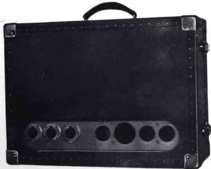
FIGURE 3—REAR VIEW OF THE AMPLIFIER-CONTROL UNIT, SHOWING CONVENIENT FLUSH OUTLET RECEPTACLES
