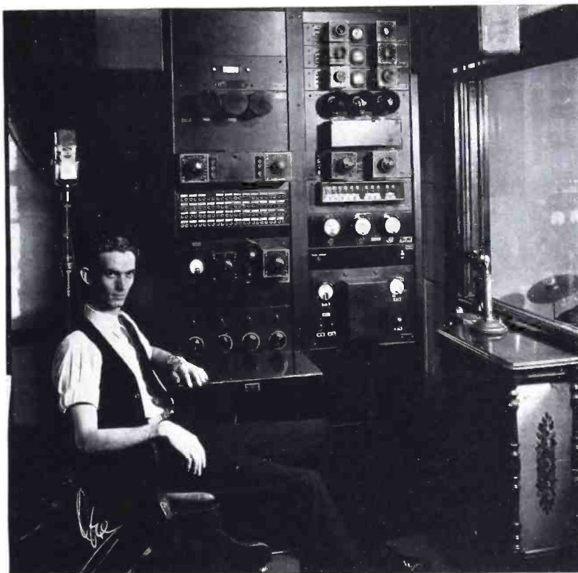
J. E. ADAMS, CHIEF CONTROL OPERATOR AT WFBC, IN THE CONTROL ROOM WHICH NOW INCLUDES AN RCA VICTOR 41-B PREAMPLIFIER, A NEW 4-CHANNEL MIXER, AND A VELOCITY MICROPHONE
