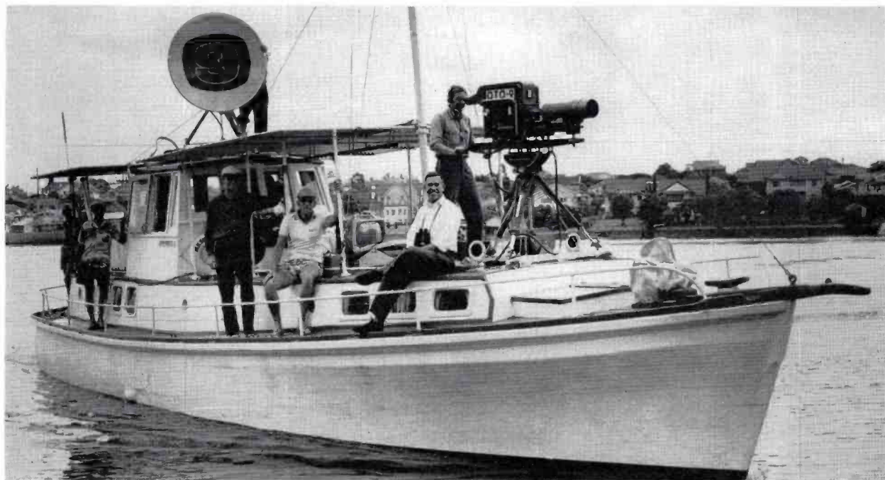
FIG. 16. A TVM-1A microwave link with 4-foot reflector and TK-31B Image Orthicon camera with zoom lens are seen mounted on a launch during a remote telecast of the 18-Footer Sailing Championships on the Brisbane River.
