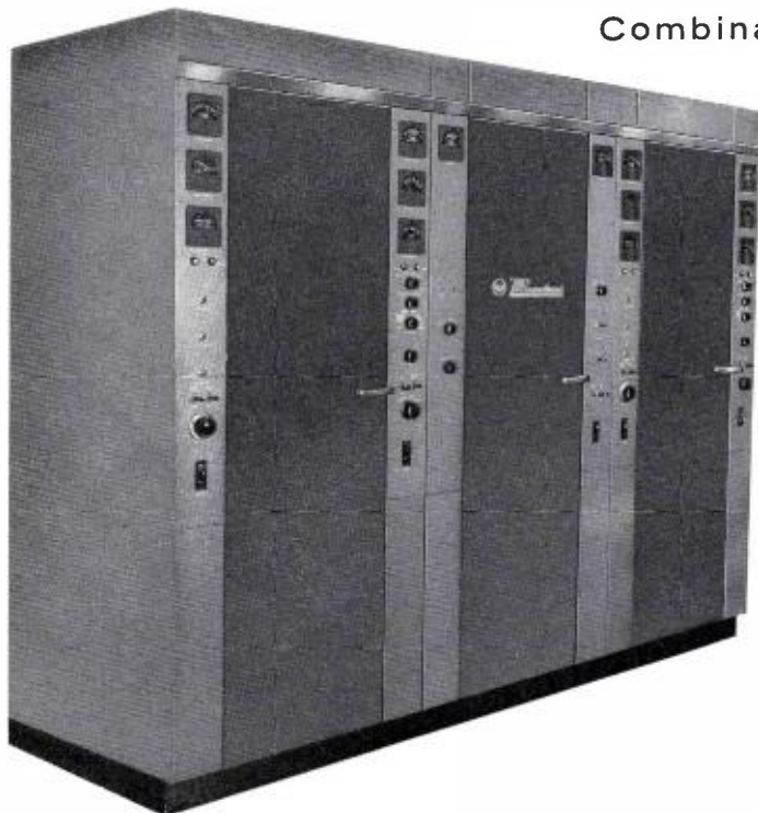
FIG. 1. The type BTF-20 is a compact three-cabinet 20-kw transmitter. It employs the RCA "Direct FM" exciter, which gives widest frequency response with minimum distortion.
