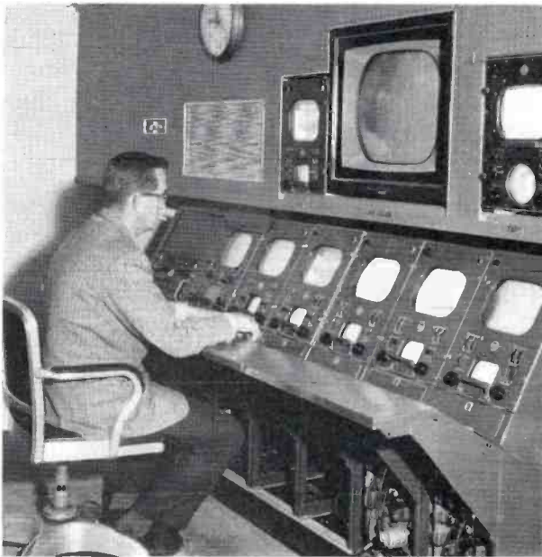
FIG. 18. Position for shading of film cameras in the master control area.
