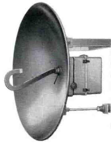
FIG. 1. Antennas less than 6 degrees off path, yet virtually no signal is obtained at receiver.
