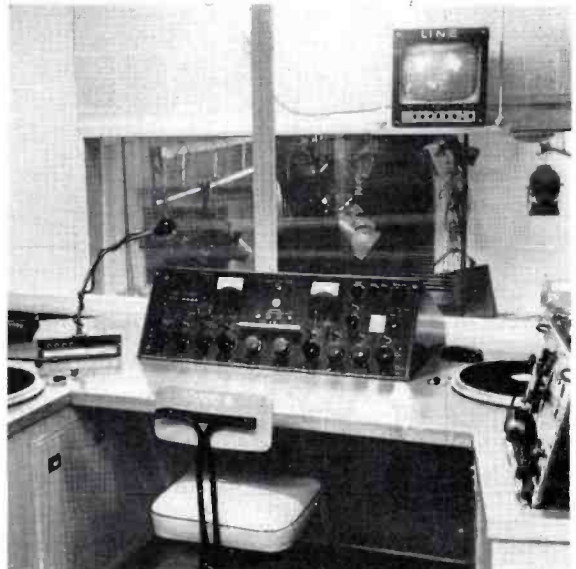
FIG. 10. The BC-6B console in the Studio B audio control room is sometimes supplemented by a four channel auxiliary mixer (not shown).
