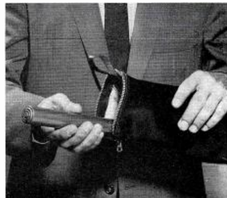
FIG. 3. The complete microphone-amplifier combination—together with earpiece, jack and 25-foot cable—is carried in a small zippered bag.
