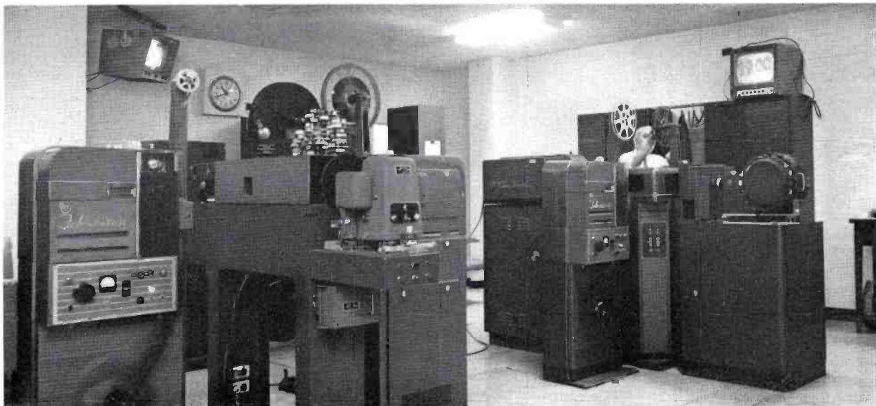
FIG. 14. Film room has two monochrome systems similar to one at left, and one color TV film system (right).
