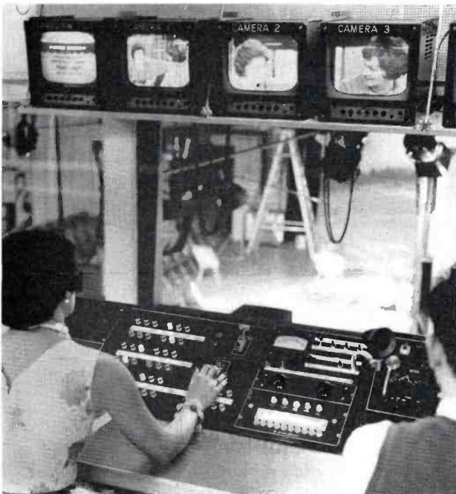
FIG. 9. The control panels for TS-40 switcher and special effects system are shown in the Studio B control room. The panel above the special effects selector includes camera intercom and studio talkback facilities for the technical director.
