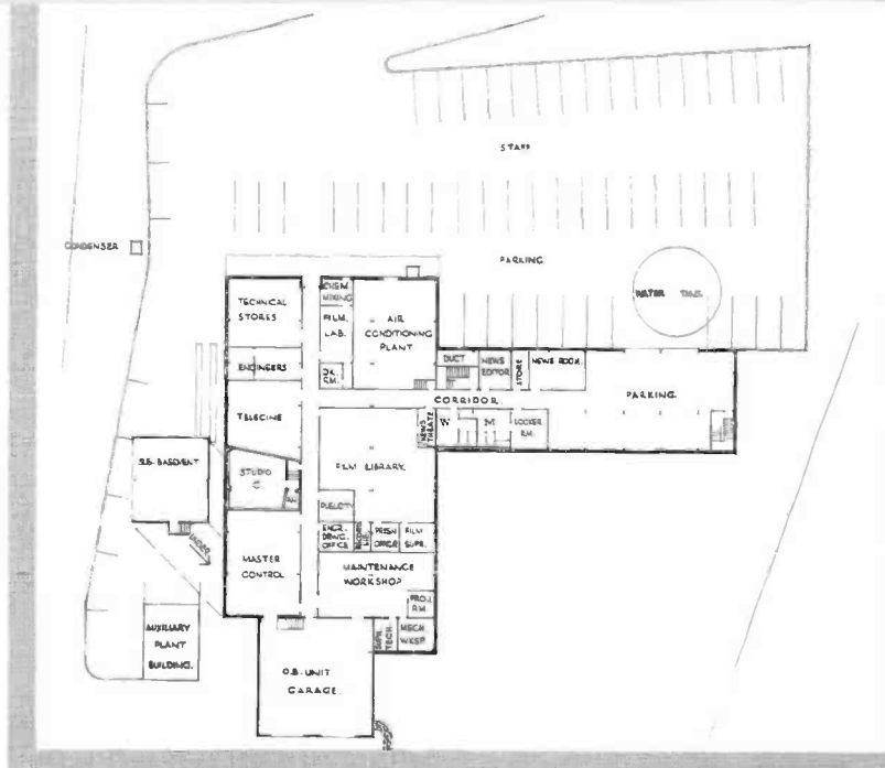
FIG. 4. The layout of the Central Technical Area can be seen clearly in the architect's simplified basement floor plan.
