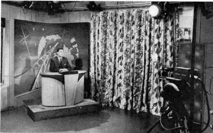
FIG. 11. Studio C is 21 feet by 21 feet and is used for the presentation of News and Weather Bulletins together with simple live commercials and interview-type programmes. This Studio is equipped with a TK-21 vidicon camera used in conjunction with a zoom lens. The camera and lens have complete remote control of pan, tilt, focus, iris and zoom. Preset lighting and the special camera facilities allow for unattended operation in this Studio.
