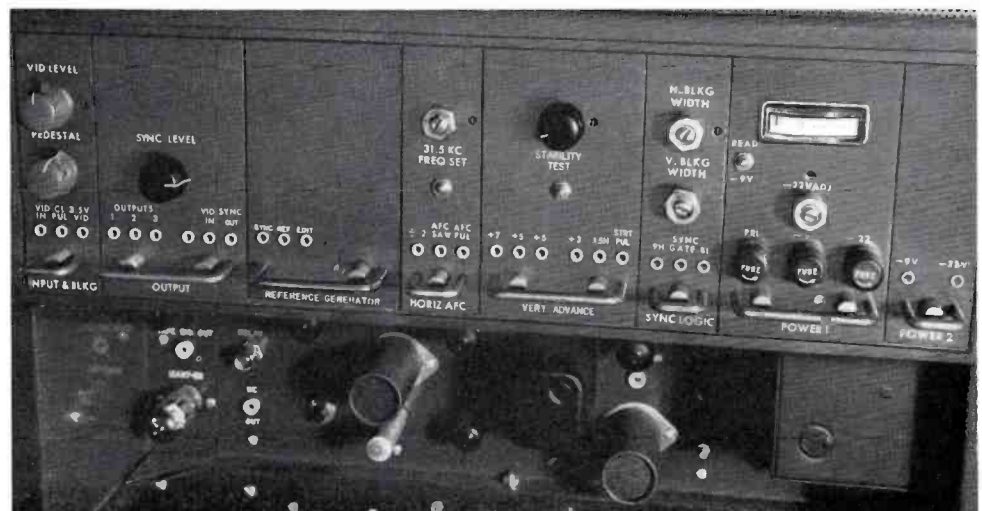
FIG. 5. The sync separation function is contained in this transistorized reference generator module, third unit from the left in the processing amplifier. This module also provides reference and edit pulses.
