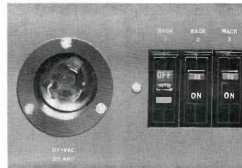
FIG. 8. Low power consumption in the TR-11 permits a single a-c power feed to be supplied to one main connector. Three a-c breakers evenly distribute power throughout the recorder.
