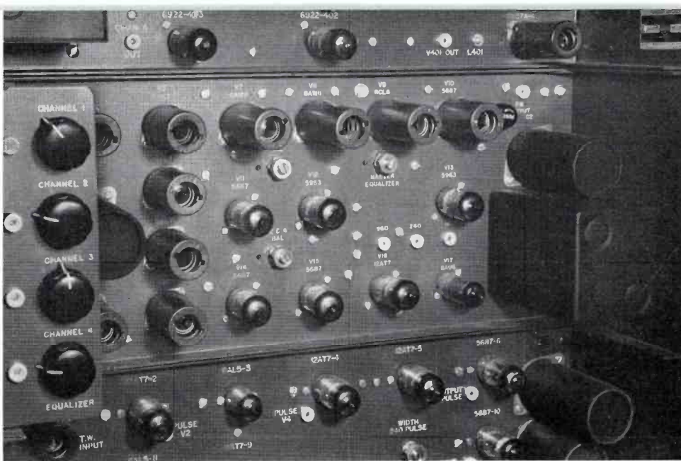
FIG. 4. This chassis incorporates the functions of both the 4 by 2 and 2 by 1 switchers found in the TR-11's senior partner, the TRT-1B TV Tape Recorder. In the re-design of this unit the sync separation function has been relegated to another chassis.
