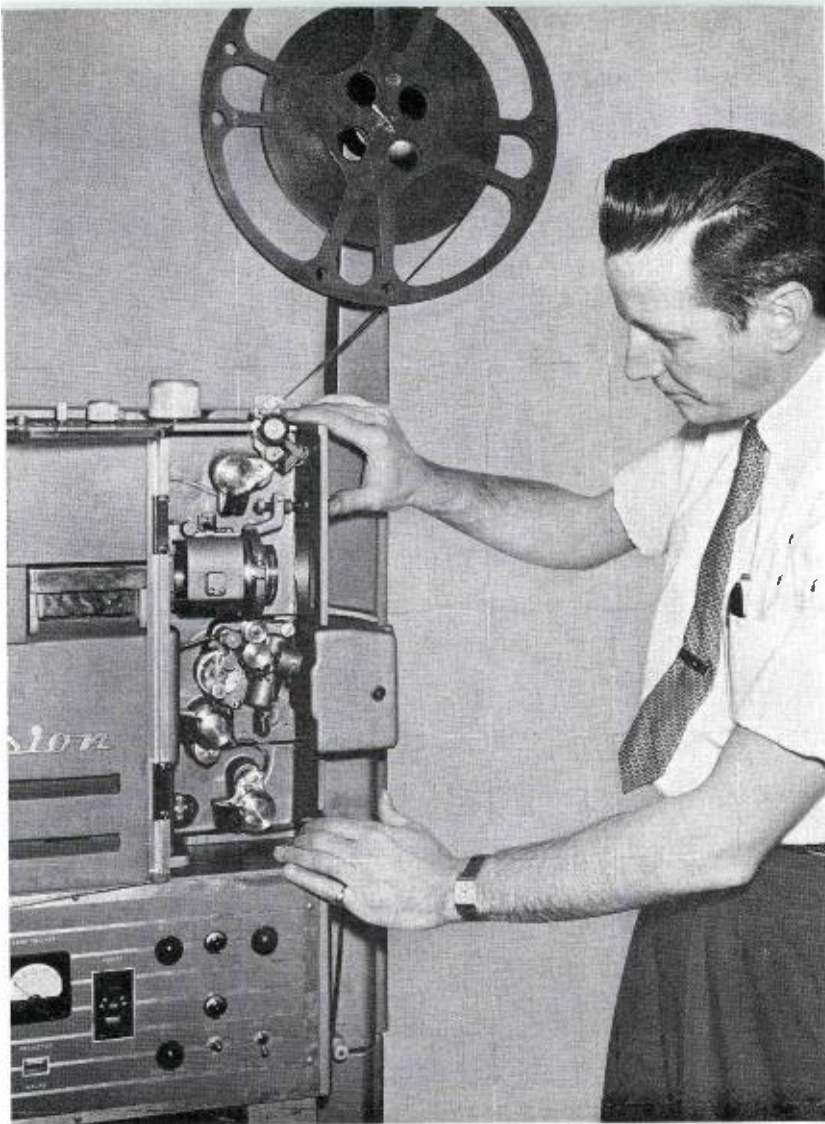
FIG. 7. A split roller is installed just ahead of the power film sprocket in place of the reel guide roller. This split roller is shown here just to the left of the operator's right hand.
