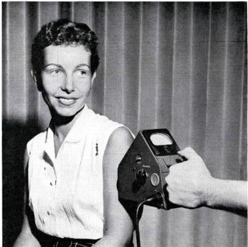
FIG. 13. A complete self-contained RCA luminometer provides excellent means of determining gray scale rendition. Direct readings can be taken as shown here after the luminometer has been calibrated on a white card for 85 percent reflectance.
