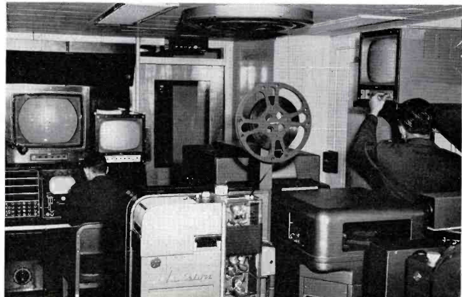
FIG. 8. The film room at SAC includes an RCA color film chain, 16mm film projector, 35mm slide projector and multiplexer. Films and slides, interspersed in briefing program schedule, educate SAC command in various fields of military knowledge.
