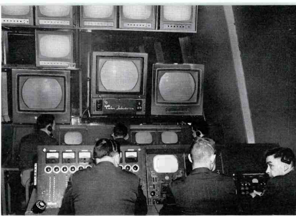
FIG. 9. Here is the well-equipped SAC TV control room. Personnel operating controls are of the Presentation Branch, Control Division, Directorate of Operations. They control cameras, and do the switching.
