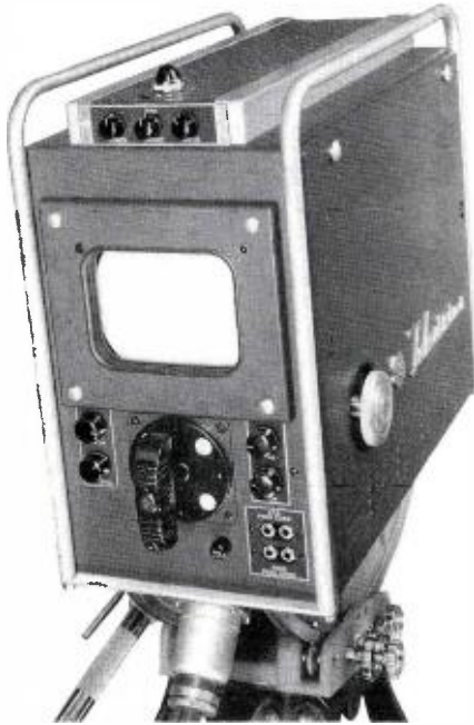
FIG. 4. Note large 7-inch viewfinder; convenient location of controls, and easy-to-grasp turret handle.
