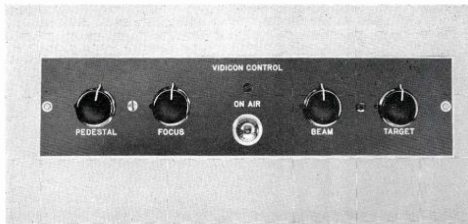
FIG. 3. Remote control panel for TK-15 vidicon camera.
