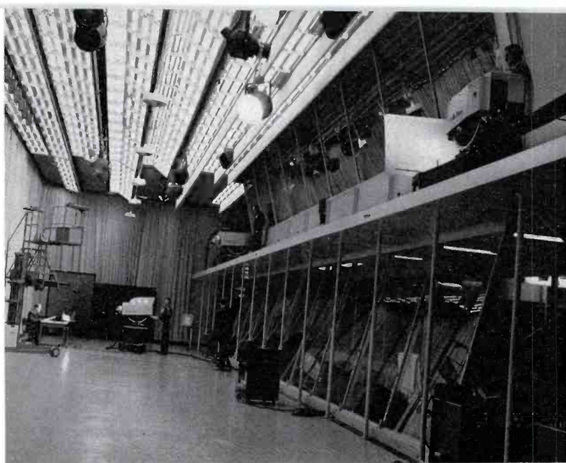
FIG. 14. A briefing emanates from the Operations Map Room. The floor camera (TK-41) is focused on the briefer. One track camera (right) is trained on a small chart supplementing the main briefing. Banks of fluorescents provide much of the lighting required for televised briefings.
