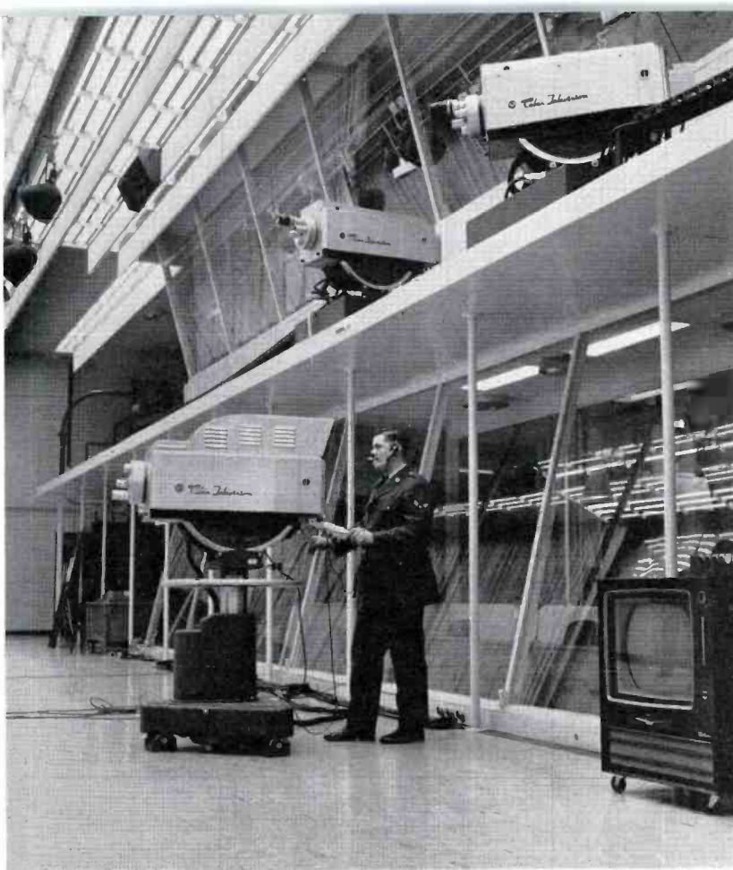
FIG. 5. Here's the battery of cameras the briefing officer faces each day as he presents operations intelligence to top SAC personnel. At top, two TK-41 Color TV Cameras can be remotely panned and tilted, moved along the 106-foot track. Third color TV camera is operated in normal manner. A fourth camera is available, and it can also be wheeled into adjacent Intelligence Room.
