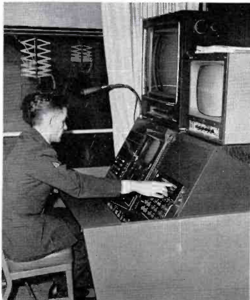
FIG. 7. Film-room operator controls film and slide output from this control console. Atop console are a 17-inch program monitor and a 21-inch on-air color monitor. Film room is in glassed-in balcony area above map room.
