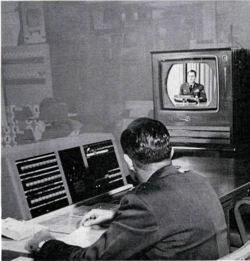
FIG. 13. View of the Operations Control Room, one of the locations receiving briefings via color television. Note RCA color TV monitor. Controller, foreground, can be put into immediate touch with SAC bases all over the world to sound the alert in case of enemy approach.
