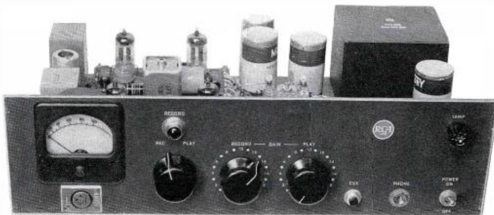
FIG. 2. This is the Type BA-51A Recording Amplifier. Note the microphone connector under the meter. The red panel light glows when the amplifier is in the record position. Cue burst is inserted with the small "cue" push-button switch.
