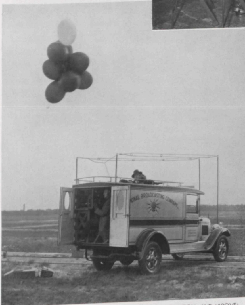
NBC RADIO RELAY TRUCK NEAR THE SCENE OF THE INAUGURATION, AND (ABOVE) CONTROL OPERATORS BUSILY ENGAGED IN TRANSFERRING OUTSIDE PICKUPS FROM ONE VANTAGE POINT TO ANOTHER.
