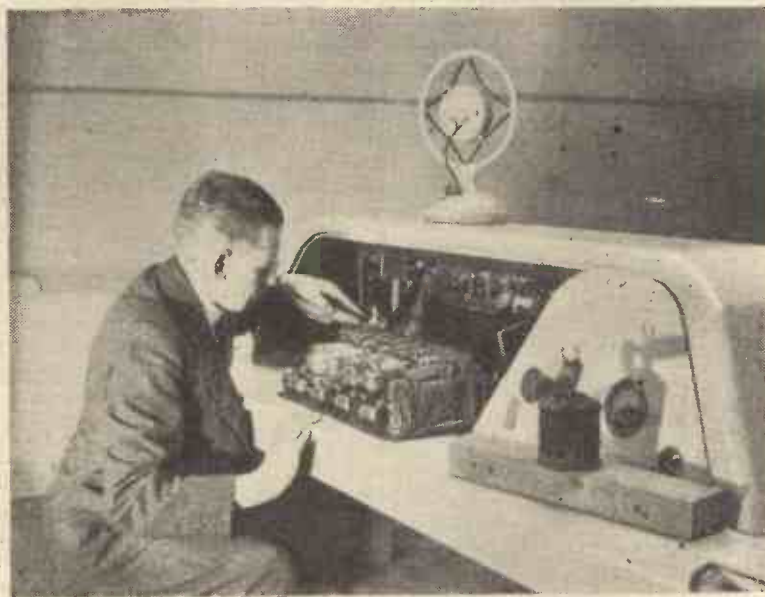
Maintenance work on one of the dramatic control panels at Broadcasting House. Systematic working is essential for tracing faults in apparatus of this nature
