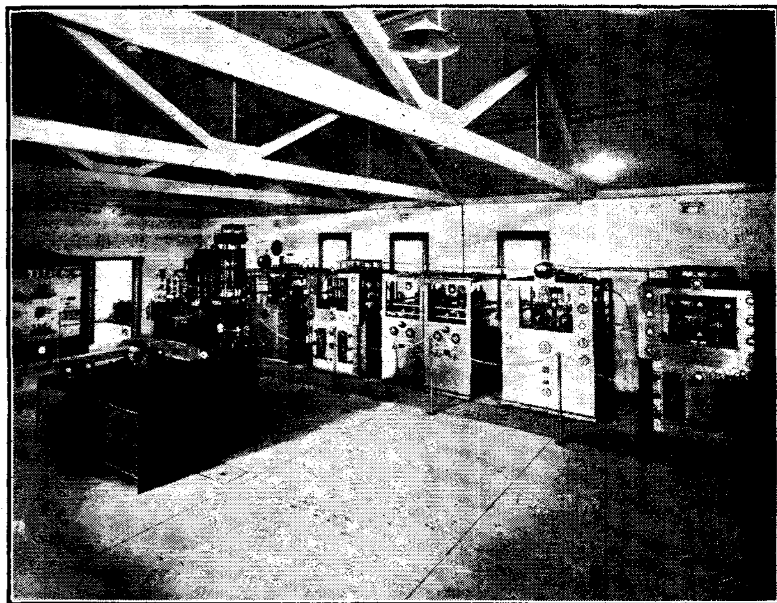
The 20 kW short-wave transmitter of VK3ME, 31.28 metres, at Melbourne, Australia
