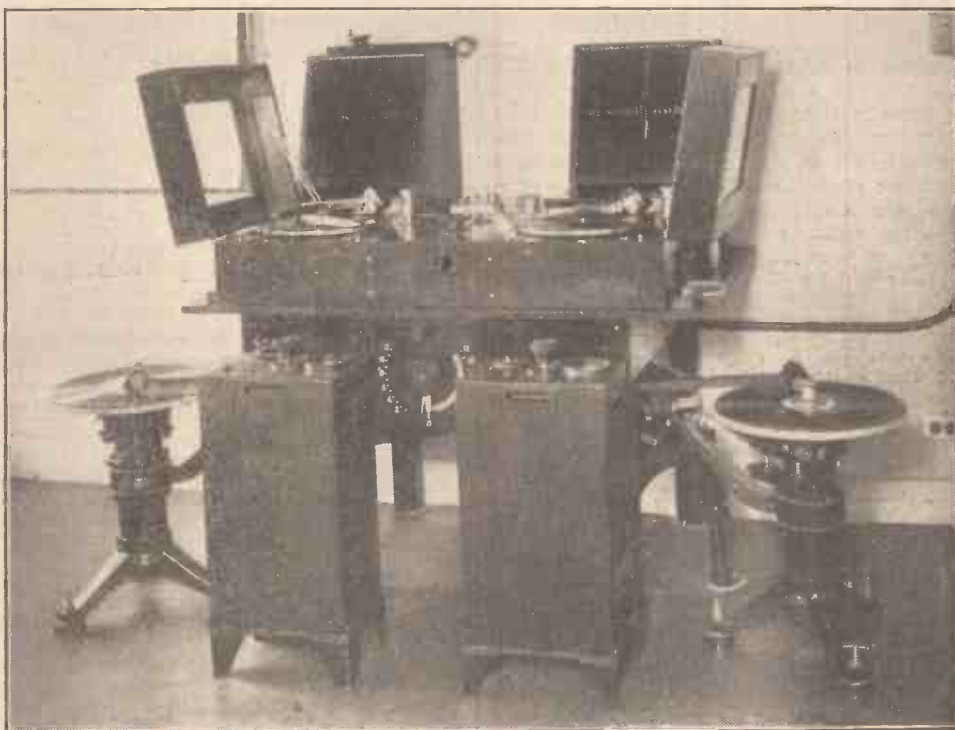
"CANNED" PROGRAMMES Apparatus at Station WOR, New York, which provides an hour's continuous transmission of an electrically-recorded programme
