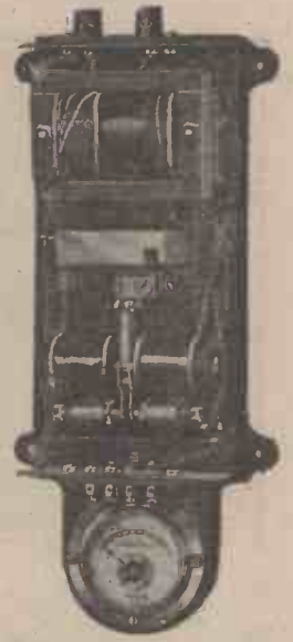
Goltone “Pendelton” Charger showing Cover removed.
