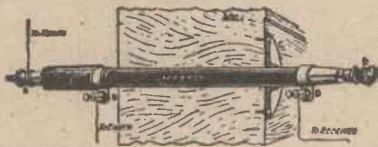
The Webb lead-in and earthing-switch.
