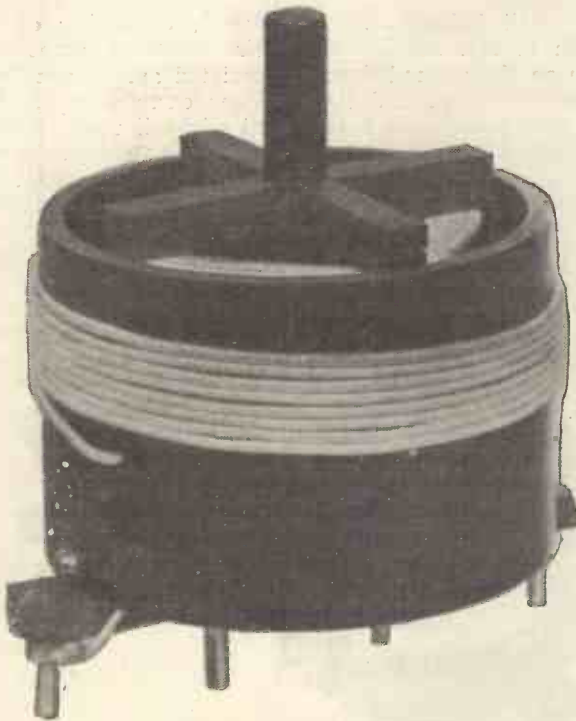
A nearer view of the aerial and secondary unit which shows that the thick wire used gives a spacing effect by virtue of its springiness.
