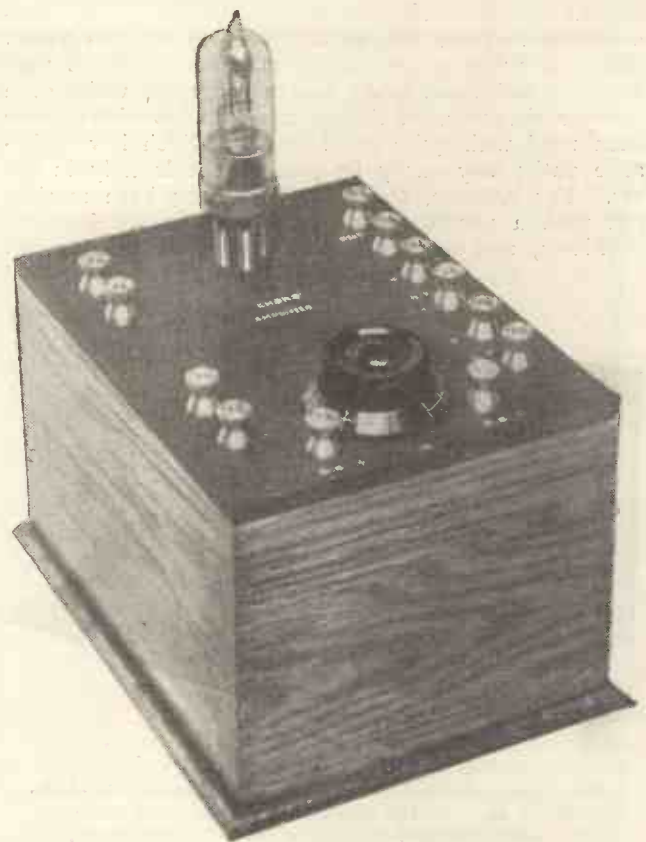
The original single-stage choke amplifier described by the author in "The Wireless Constructor," April, 1925, issue.
