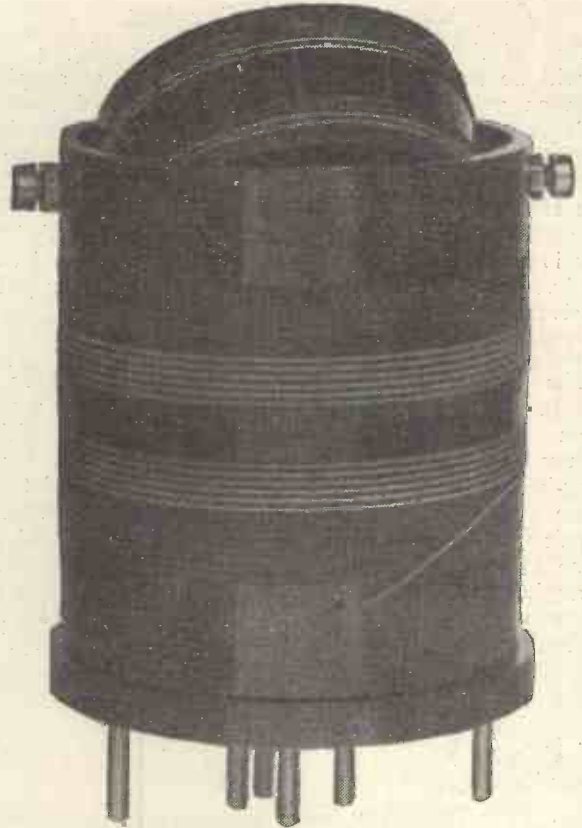
The finished coupler. Note that the turns of the windings are slightly spaced.
