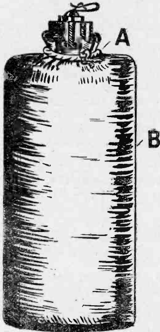
Fig. 3.—Showing how the carbon compound block may be tied up in a piece of cloth.
