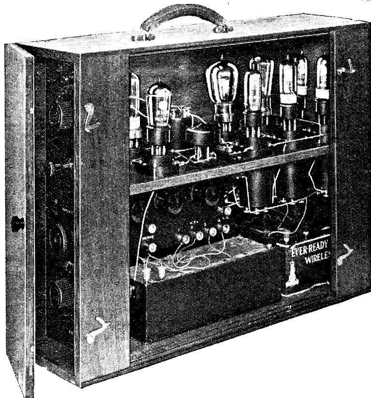
An eight-valve portable super-heterodyne receiver designed by Mr. Kendall and described in the July, 1925, issue of "Modern Wireless"
