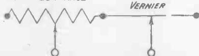
Fig. 2.—Showing the usual method of adding a vernier in series with the main resistance.
