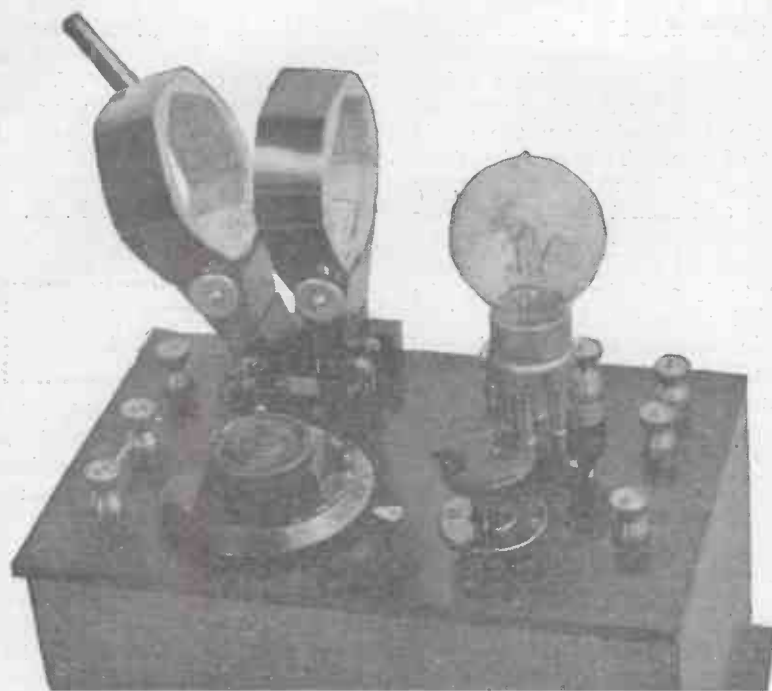
A Compact Single Valve Flewelling Receiver.
