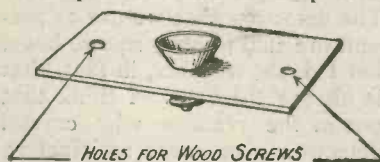
Fig. 1.—Showing method of mounting the lamp holder.
