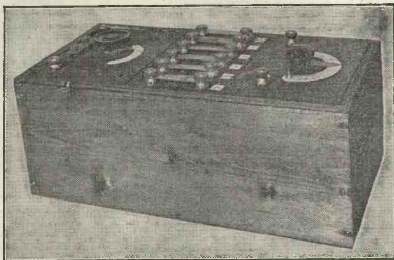
The fourth series of units comprising potentiometer, variometer and switchboard.
