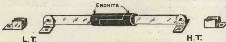
The switch shown in its correct position.
