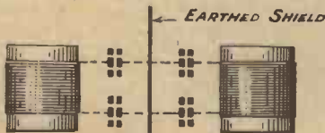
Fig. 1.—Capacity coupling between two circuits can be overcome by interposing between them a metal shield connected to earth potential.
