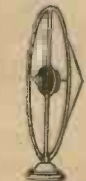
A cone diaphragm loud speaker can easily be constructed. The illustration shows one method of mounting to the "Lissenola."
