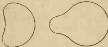
Fig. 6.—Incorrect combination of a frame and an outside aerial will give distorted polar diagrams like these.
