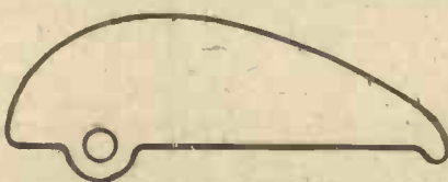
Fig. 3.—This is an outline of a plate from a straight-line-frequency condenser.
