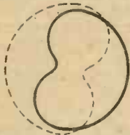
Fig. 4.—"The result of adding, if the voltages are equal, is that in one direction the signals are doubled—and in the opposite direction they are brought to zero, and the result is shown in this curious so-called heart-shaped diagram."
