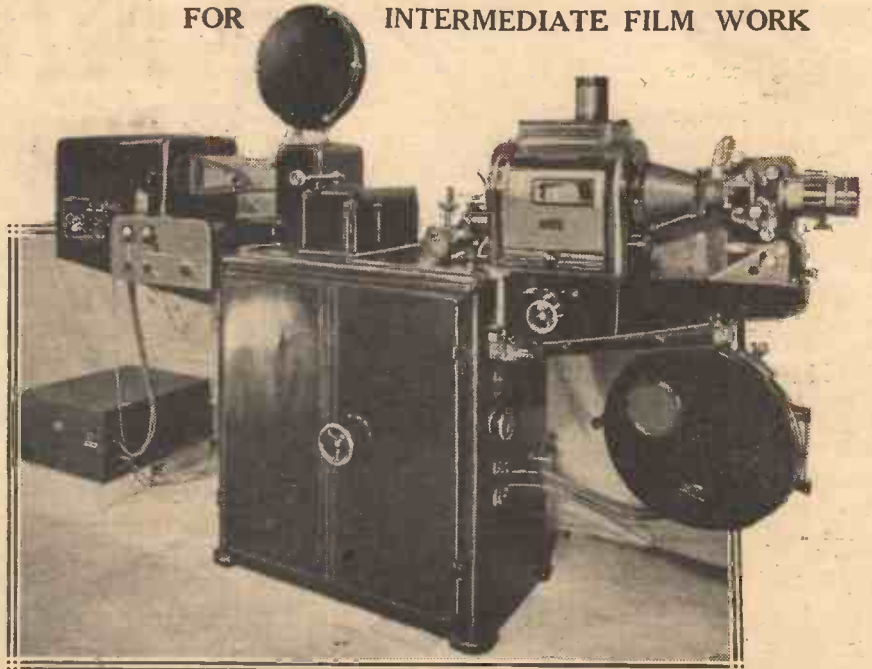
The Fernseh A.G.'s intermediate film television projection receiver which produces a picture about the size of those normally seen on a cinema screen.
