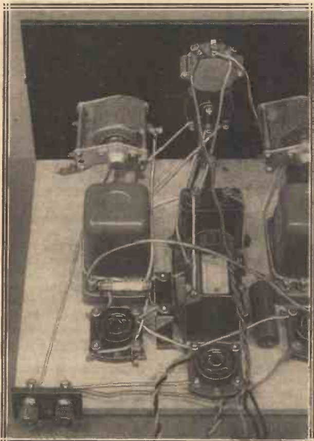
The detector and output valve holders and the detector tuning condenser and coil can be seen in this photograph. The potentiometer on the panel is for the control of the variable-mu S.G. valve.
