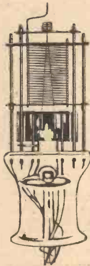
The sketch above contrasts strikingly with that on the right. Above we have the electrode arrangement of a battery double-diode triode. Note the spring tension for the filament. Compare it with the crude hand-made assembly of the "R" valve of years ago, shown in the other sketch.
