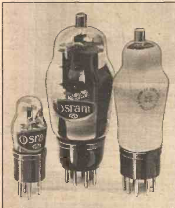
A trio of 1935 valves. On the left is a double diode, the centre one is the D.N.41, a double diode and steep slope output pentode; the right-hand valve is a multi-mu screen pentode with double diode inside.
