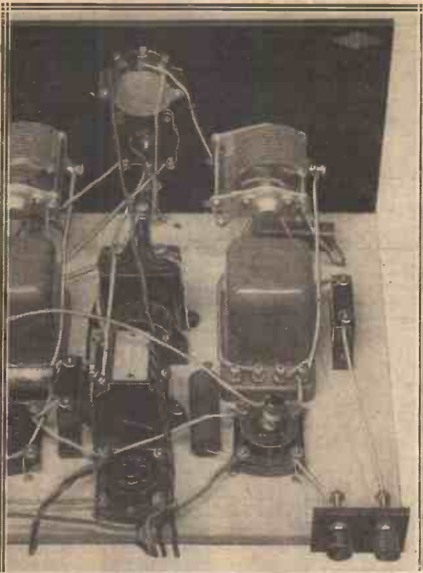
This photograph shows again the output valve holder and the L.F. transformer but includes the S.G. stage of the "Easy-Build" Three. The S.G. valve holder is not as unusual as it at first appears, the "centre terminal" is merely the top cap fitting for the S.G. valve.
