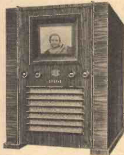
The Lorenz-Von Ardenne television receiver shown at the German Radio Exhibition. The size of the picture is about 7½ ins. by 9 ins. A four-stage superhet is used for vision and a three-stage reaction receiver for sound.
