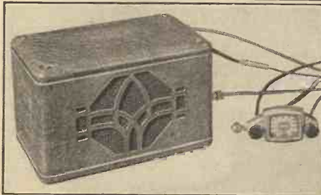
This photograph shows the whole of the Philco car radio installation, apart from the aerial. Note the neat controls for steering column or dashboard mounting.
