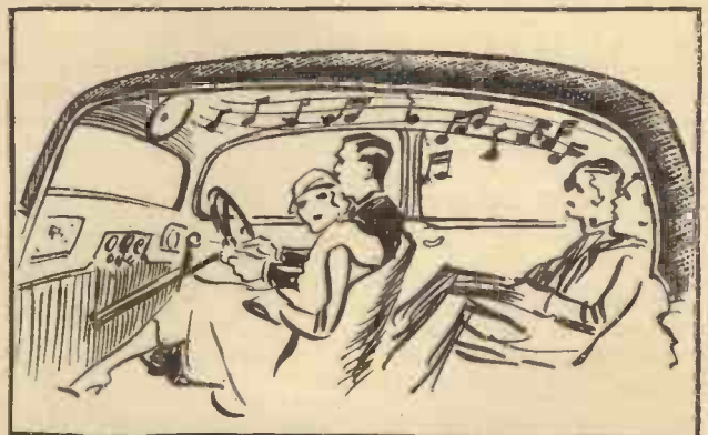
If it is possible to fit the loudspeaker above the windscreen, the results will be much better from the point of view of passengers in the rear seats than if it were under the dashboard.
