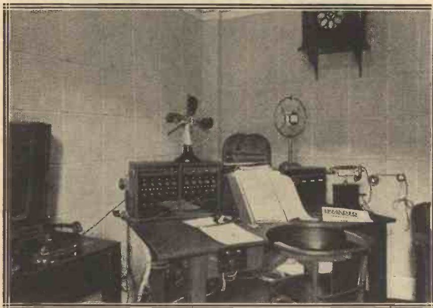
An interesting corner of the announcer's studio at Polski Radio, Warsaw. Note the special sound-absorbing walls, and how the desk is cut away to facilitate the reaching of the switches. On the left is a gramophone turntable and pick-up.
