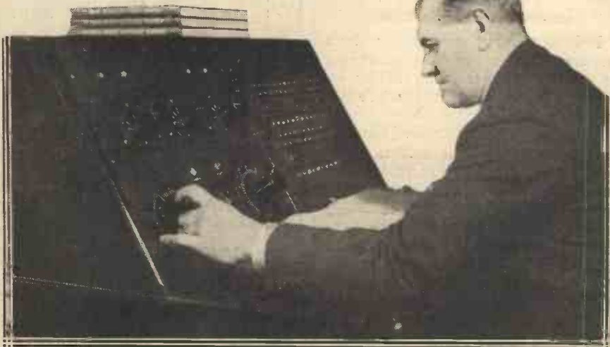
Mr. Askew at one of the Musical Control desks at Broadcasting House. The modulation meter mentioned in the article can just be seen to the right of the hand.
