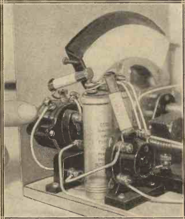
A CLOSE-UP VIEW of the volume control which controls the bias of the screen pentode valve, and thereby determines the strength of reception.
