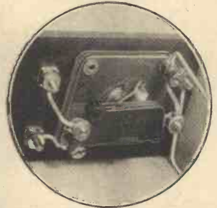
A CLOSE-UP of the two aerial terminals and the two aerial series condensers—one fixed and the other a .0005-mfd. variable.
