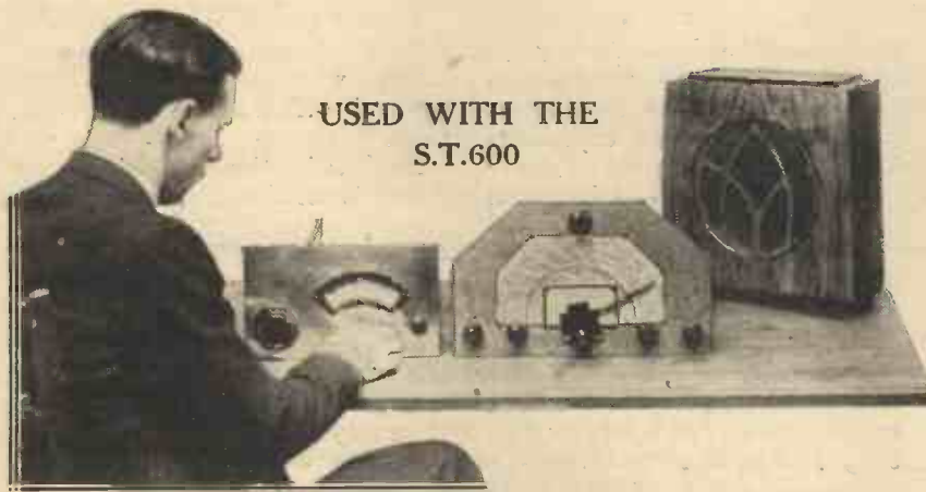
TUNING THE HEXOVERTER for the reception of short waves in conjunction with the S.T.600. The "600" is tuned to a high reading on the long waveband.
