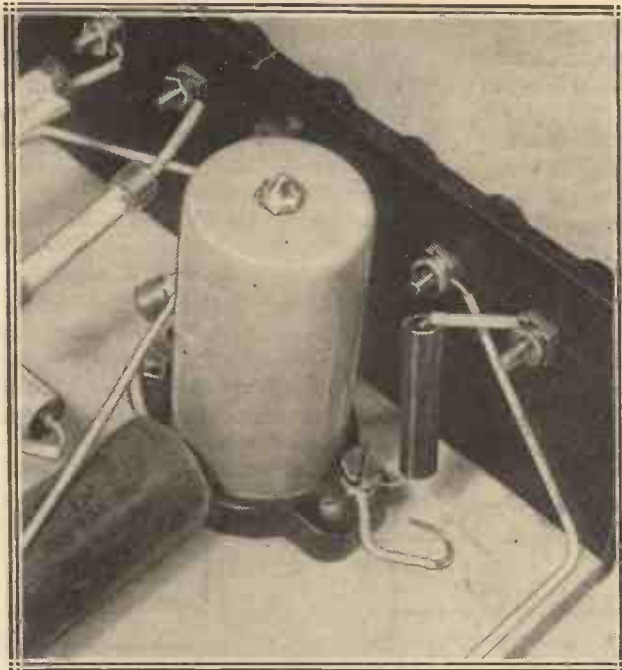
A HIGH INDUCTANCE H.F. CHOKES is essential for the anode circuit of the 210 VPT valve in the "Hexoverter." This photograph shows the choke in position, with the lead for the cap terminal of the valve attached to one terminal of the choke.
