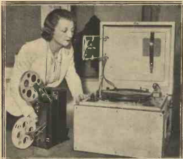
A special amplifier and microphone equipment that has been produced for the benefit of home cinematograph users. It is intended for those who wish to introduce music or a running commentary as accompaniment to the silent films that are used in home projectors.
