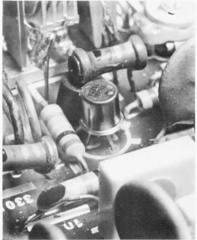
Unwanted oscillation at u.h.f. may be cured with a ferrite bead over the lead of the oscillator output capacitor.
