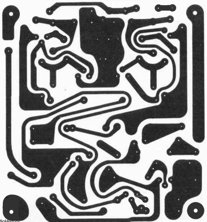
Fig. 8. Layout of suitable printed-circuit board, actual size. (Courtesy Radford Audio Ltd.)
