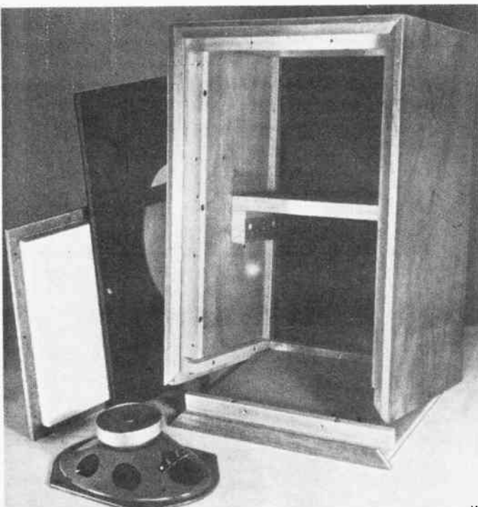
Components of cabinet, showing removable base, and the elliptical loudspeaker unit.
