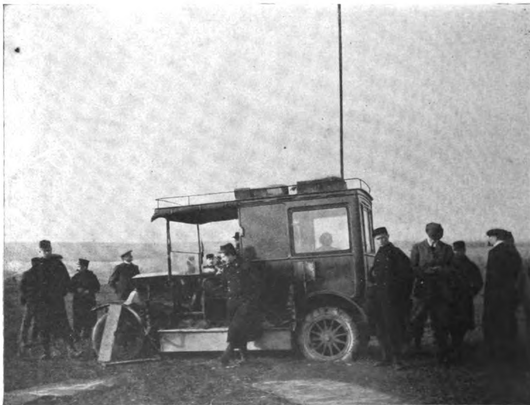
This station, which was thoroughly tested by the Belgian government, is so arranged that it requires but twenty minutes to erect the mast and establish communication.
