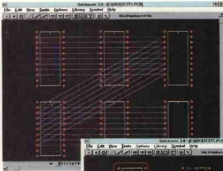
A bus structure on a small memory array was used to exercise the autorouter. This is the rat's nest showing the desired connectivity.
