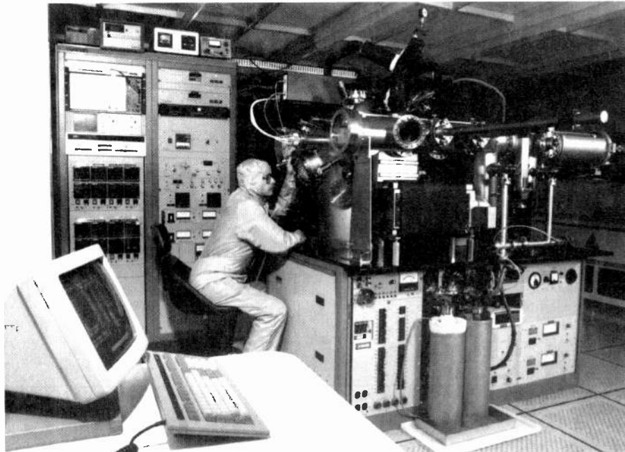
GEC Plessey's Caswell GaAs wafer production line for high volume microwave devices. Plant manager Fred Myers claims device yields up to 80 per cent on its 3in wafers. The picture shows molecular beam epitaxy equipment used to grow further semiconductor layers on the GaAs wafers.
