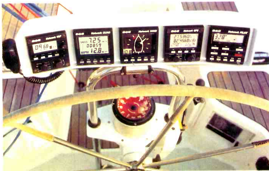
Integration at the helm: Self-contained instruments, linked together to talk to each other are the basis of Brookes & Gatehouse's Network system. The pod contains, from left: VHF; Quad (speed, log, timer, depth); wind; GPS; autopilot. Instruments can be easily switched as new facilities – perhaps DGPS – become available.
