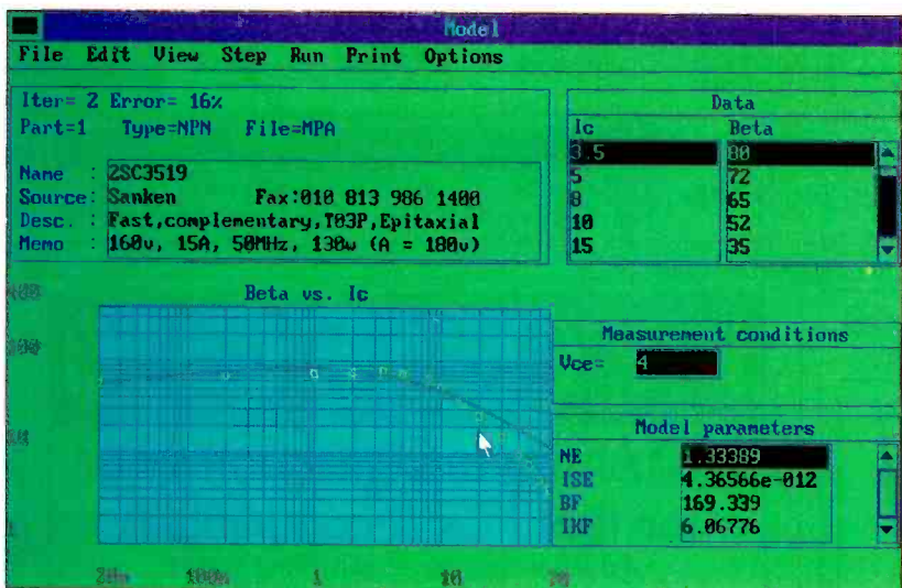
Fig. 6. MC4's auxiliary MODEL program. After entering data into the upper right table, pressing F10 prompts an optimisation routine to fit a curve to data (lower left), which can immediately be checked against the data sheet. More interpolation data and iterations will improve the fit of the h_{fe} vs I_c curve, at the high current corner (IKR). Many parametric curves show less inflexion and typically reach 10% curve-fit accuracy (indicated in top left box) with only six or so data points and two iterations.
