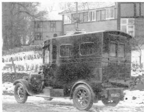
1927 Post Office patrol van, supposedly for the purpose of locating oscillating receivers, but also useful for tracking unlicensed transmitters. The frame aerial on the roof of the van was rotated by the large wheel within to take bearings.
