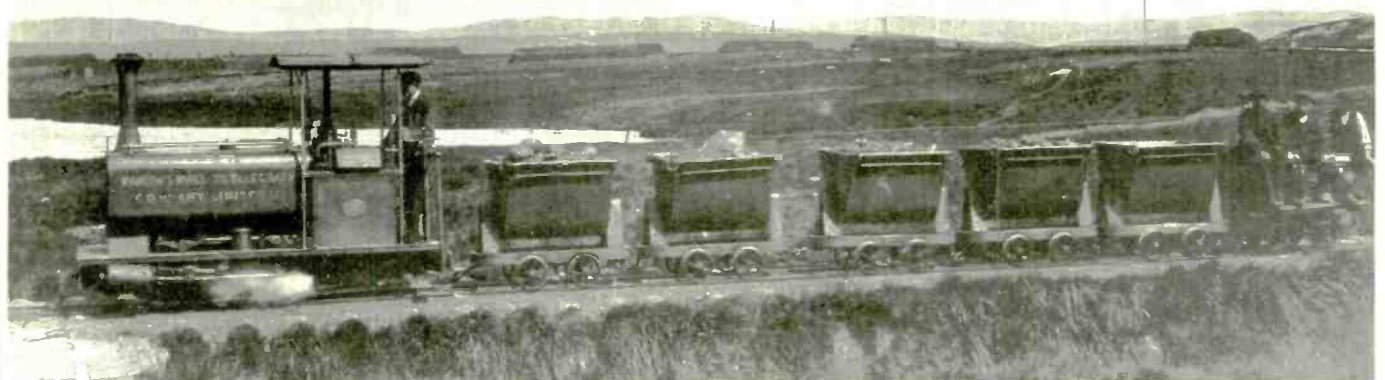
Peat train for the generators. The Clifden station used a steam engine set to charge a 6000 cell battery.
