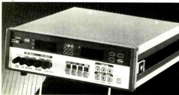
The LCR815 LCR meter from Flight has selectable test frequencies of 120Hz and 1kHz
