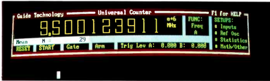
Fig. 2. Virtual front-panel layout of the GT200.
