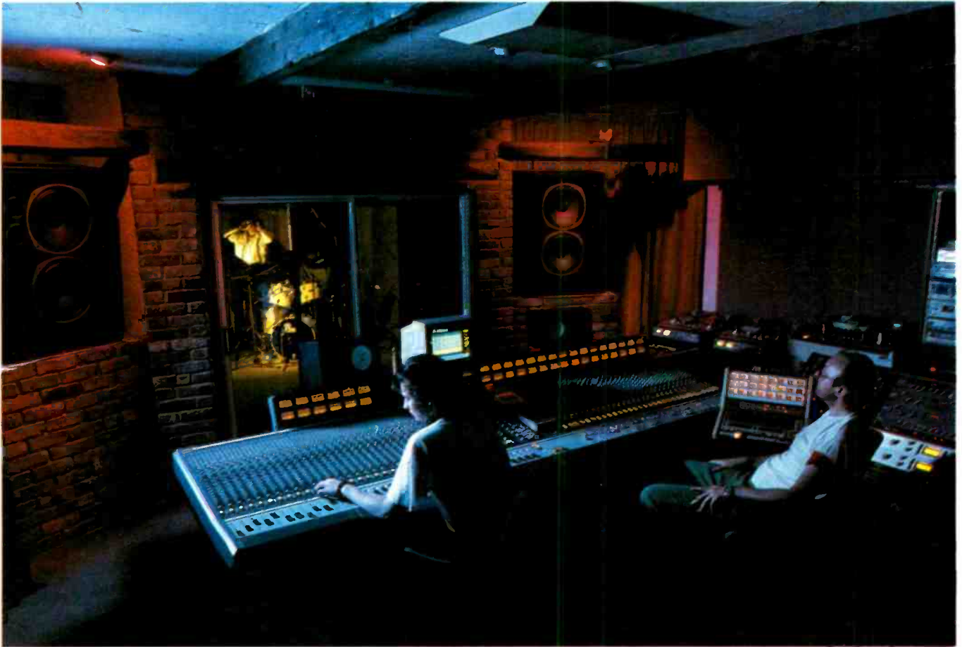
Fig. 2. Soundcraft 32000 recording console at Black Barn studio, Ripley, Surrey. Desk is an analogue design, but is used with multitrack digital equipment.
