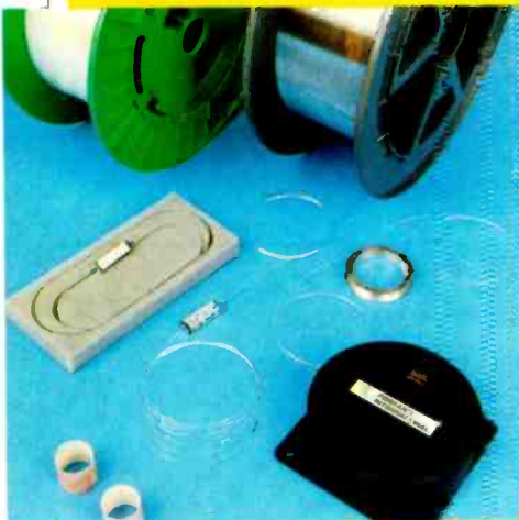
Ferranti fibre-optic gyroscope, with a selection of components. Small rectangular component is a coupler.
