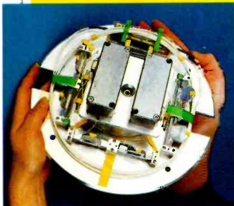
Demonstration model of FOG. Source and detector are in separate die-cast boxes, with coil below. Three polarisation controllers and an integrated-optic phase modulator (top) are shown.
