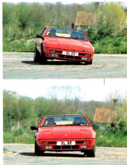
Lotus 1988 sports cars without (top) and with (bottom) real-time adaptive suspension.
