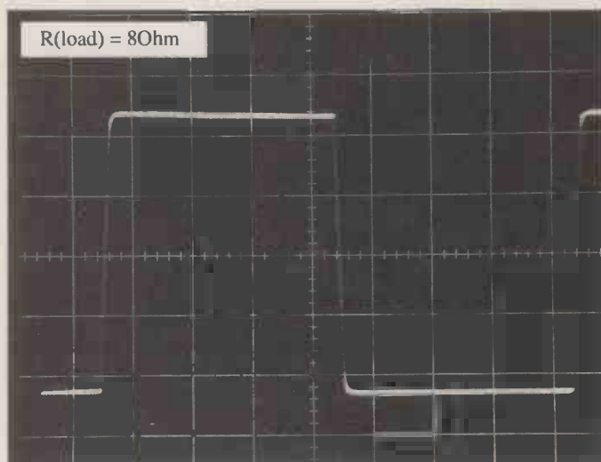
Fig. 12. These photographs of the square-wave response demonstrate the amplifier's stability. On the left, load is 8\Omega , on the right, 1\mu\text{F} .
