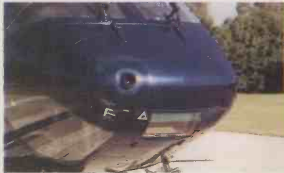
Electronic eye... A laser radar capable of warning helicopter pilots of obstacles such as overhead cables has been developed by Dornier. Objects as small as five millimetres thick can be detected from a range of several hundred metres, giving pilots plenty of time to avoid the obstacle.
