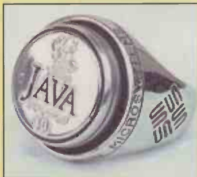
Fig. 1. Java on a button. Dallas Semiconductor's iButton is a computer chip housed in stainless steel. It can be worn by a person or attached to an object for up-to-date information at the point of use. Each button holds a guaranteed-unique registration number engraved in the silicon. Some buttons have memory to store typed text or digitised photos; information can be updated as often as needed with a simple, momentary contact. Some buttons even have a real-time clock, temperature sensor or transaction counter.
