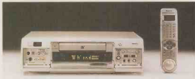
Panasonic's NV-DV10000 Digital Video Master VCR has a detachable wireless edit controller that operates the VCR and camera, etc. It also has PCM audio together with IEEE1394 (i-Link or Firewire) for high speed transfer of digital video to a pc and RS232C for transferring digital stills to a PC. In addition to the normal analogue connections, there's a 5-pin connector for S-VHS/VHS, 8mm LANC.
