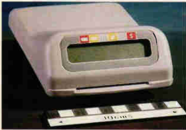
The GEC on-vehicle smartcard unit, also used in DETR trials, operates on similar principles to the Bosch unit.
