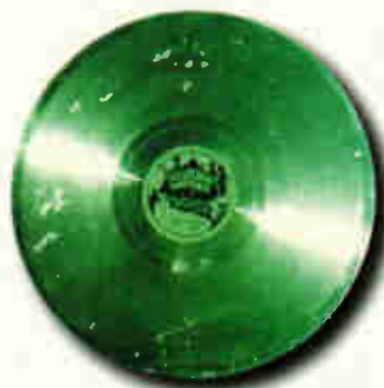
Fig. 1. An enthusiast made the earliest known 'home video' recording in 1933 onto an aluminium disc intended for audio. The extensive damage caused by corrosion shows up as light patches on the disc surface.
