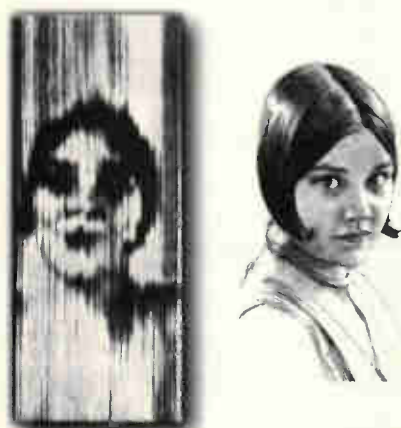
Fig. 6. One of the very few existing off-screen photographs from the thirties of a live received transmission. This high contrast picture of Betty Bolton was a long exposure directly from the mirror-drum display onto a photographic plate. The picture on the right shows Betty to be more attractive than the photo indicates.
